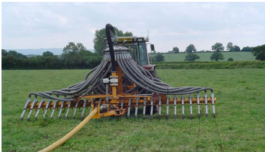
Plate 3: Shallow injection slurry applicator
