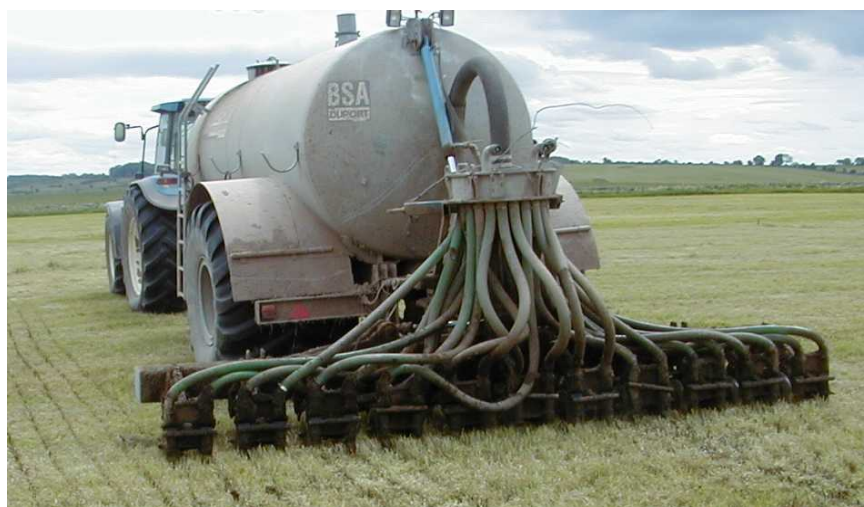
Plate 3: Shallow injection slurry applicator
