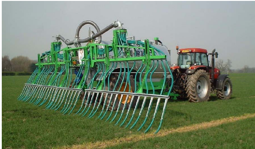
Plate 2: Trailing shoe slurry band spreader
