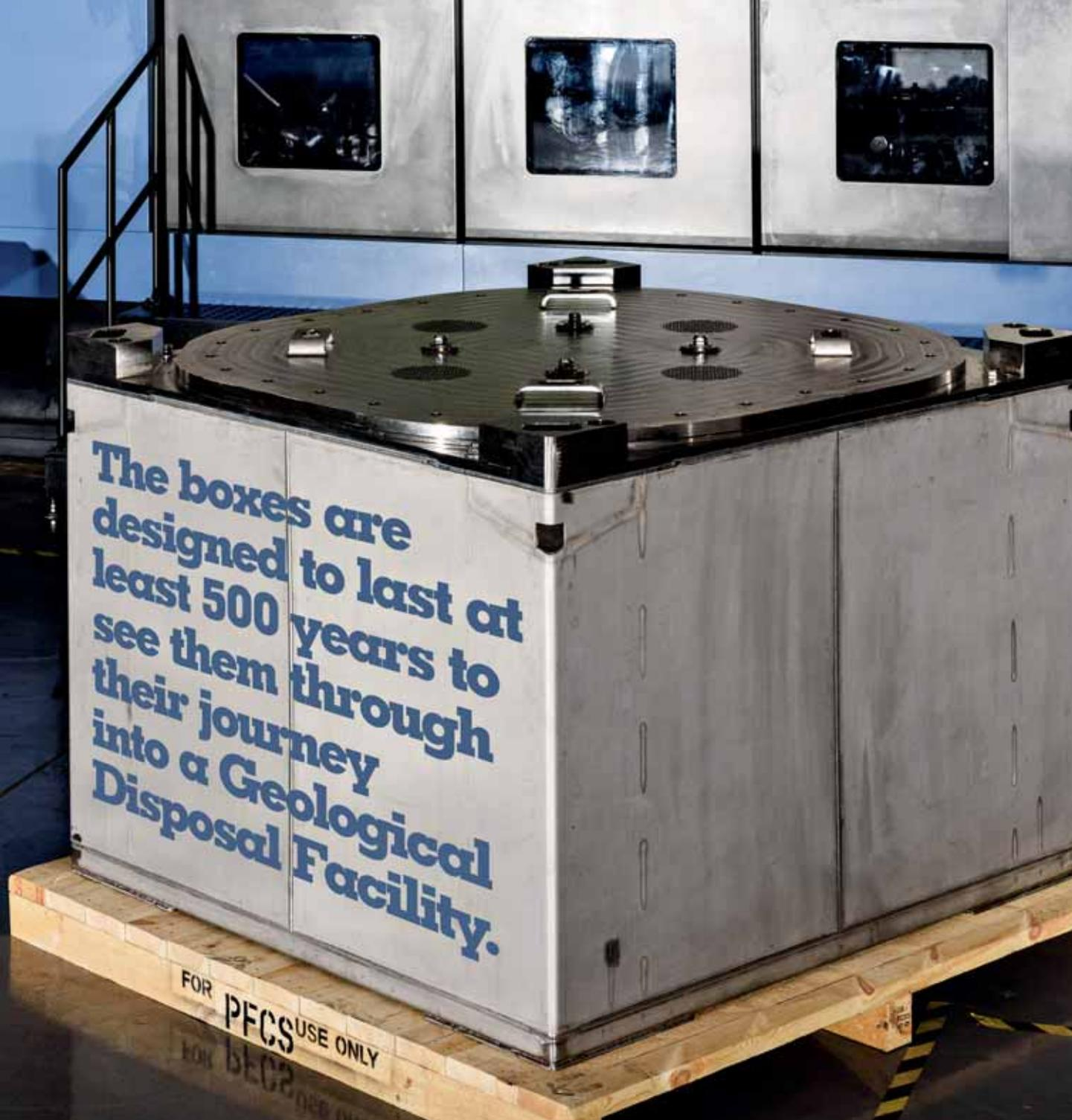
Thanks to an innovative new approach in how we treat and store the waste, retrievals from the Magnox Swarf Storage Silo have been accelerated. There will be a new contract competition starting in 2018 to make these 3m<sup>3</sup> boxes, but some are already in the production pipeline so we can start getting waste out in 2019 before the big box manufacturing contracts kick in and the main facility to take the waste, the Box Encapsulation Plant which is currently under construction, opens in 2021.
