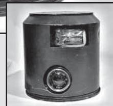
**In 1965 the team at Calder Hall deployed their own version of AVEXIS to inspect the inside of one of the station's reactors. Pictures left to right are: Percy Gill, George Buckley and Bill Robertson. Inserted: the photography equipment used to inspect a reactor vessel.**
