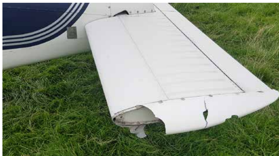
Figure 2 Damage to tip of left stabilator
