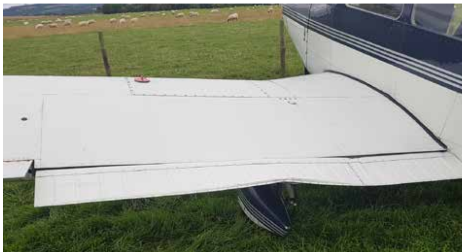
Figure 1 Damage to left flap
