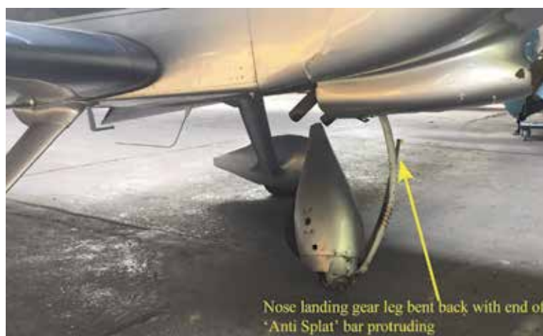
Figure 2 An 'Anti-Splat' kit was fitted to the nose landing gear
