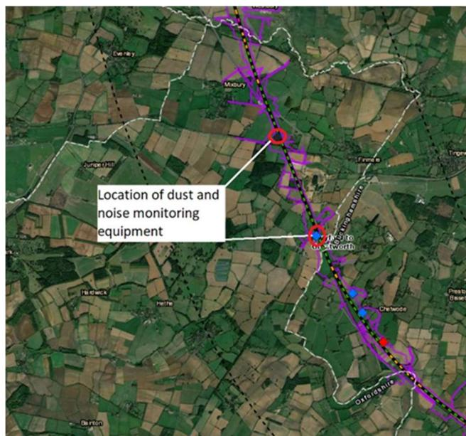
Figure 4: Location of noise monitoring equipment
