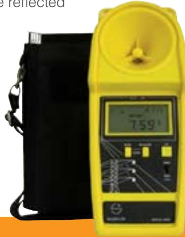
To account for the fact that speed of sound varies with temperature, a temperature sensor, mounted at the front of the instruments, senses the actual air temperature, and automatically compensates.
