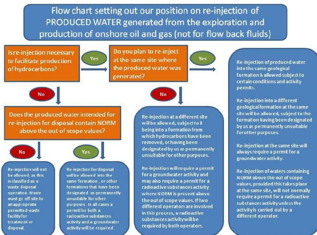
**Figure A.1 Environment Agency's draft approach to reinjection of produced water**
