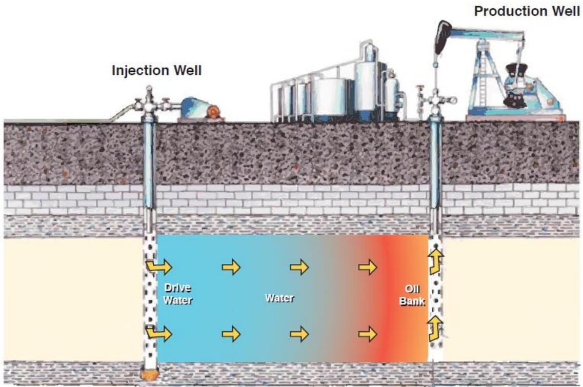
**Figure A.6 High level overview of the reinjection arrangement**
