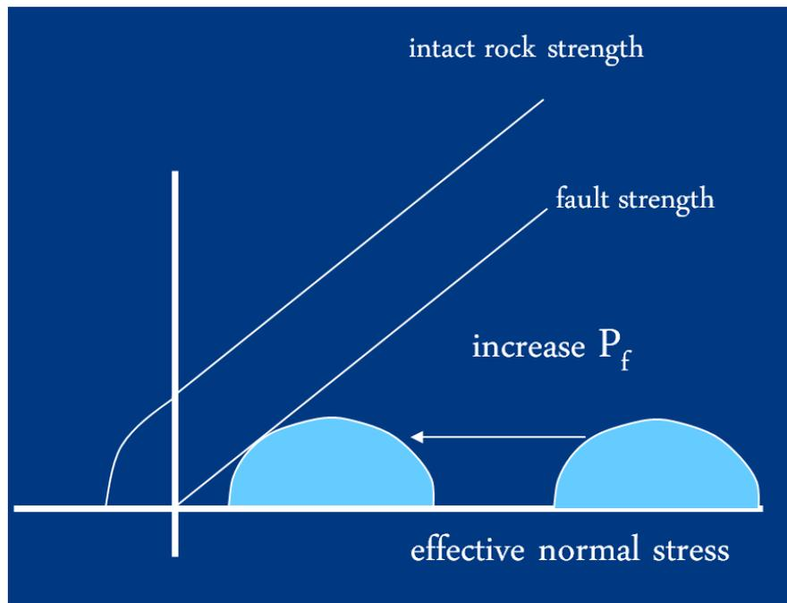
**Figure A.9 Influence of stress perturbations on the stress field inducing Coulomb failure represented by Mohr's circles of stress**
