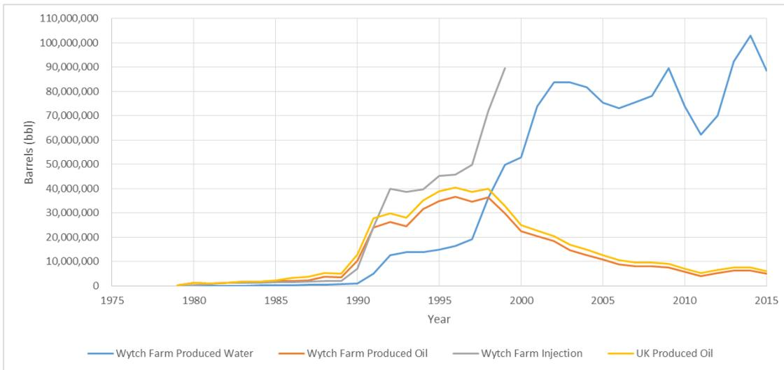
**Figure A.3 Onshore oil production showing Wytch Farm contribution to UK oil production, and volumes of injection and produced water**
