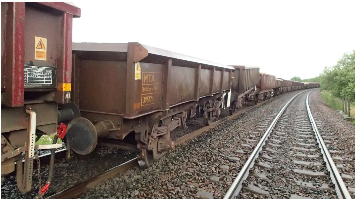
Figure 9: The derailed wagons within train 6K06
