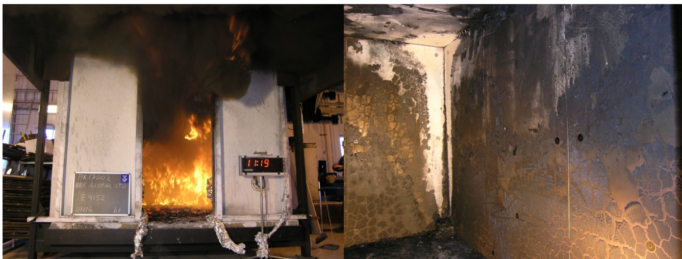
Figures D2 & D3 - Approaching flashover and post test interior photos E4152.
