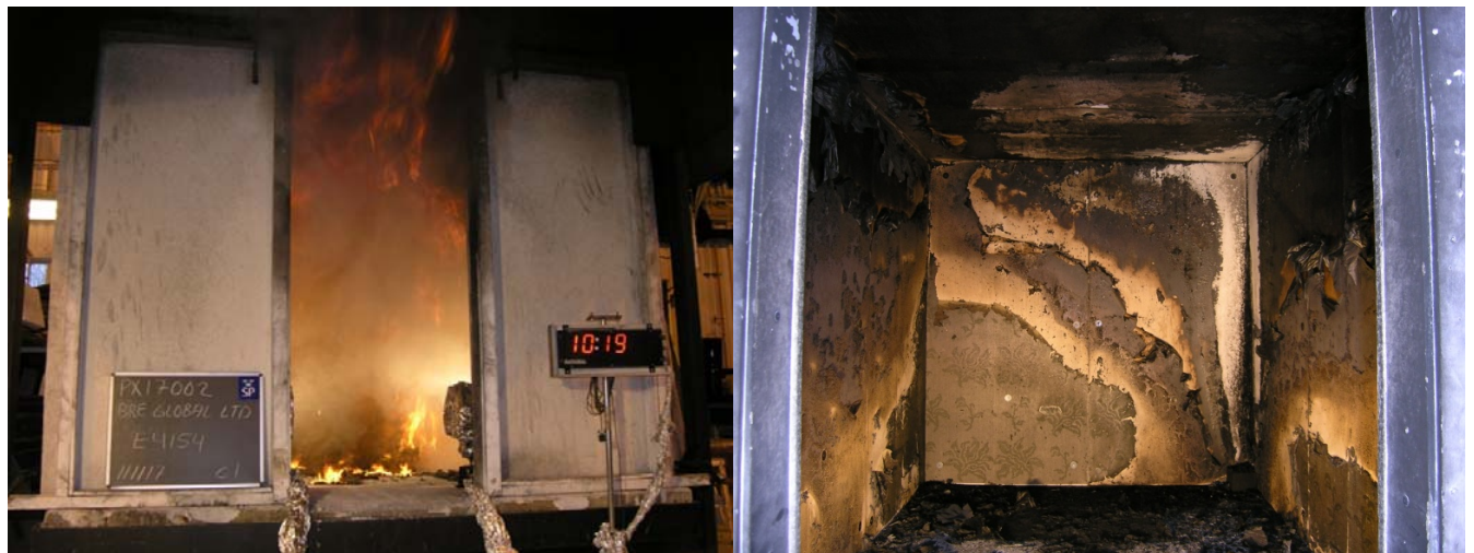
Figures D5 & D6 - Approaching flashover and post test interior photos E4154.
