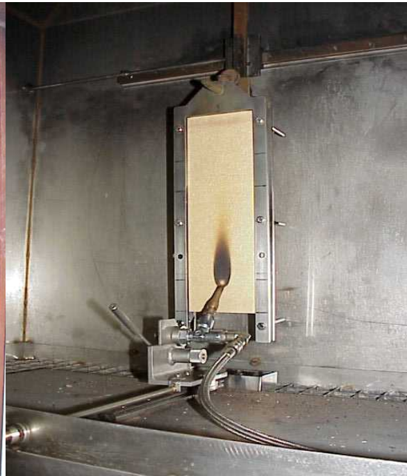
Figure 2. ISO 11925-2 Small flame test.
