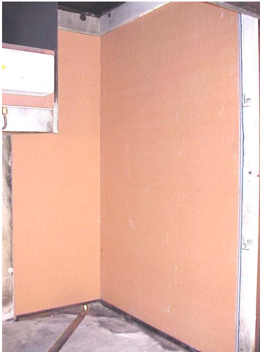
Figure 1. EN 13823 SBI test specimen
