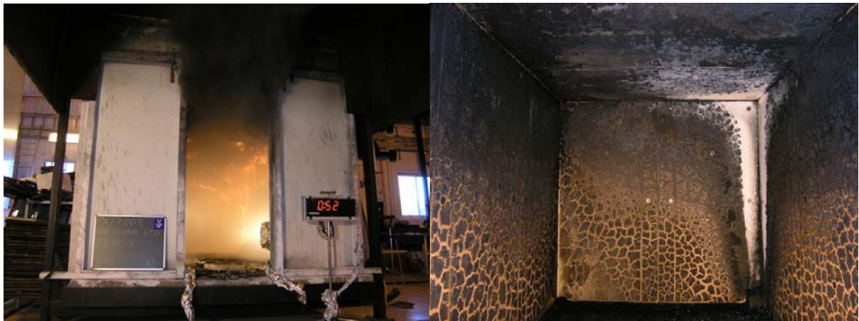
Figures D8 & D9 - Approaching 1 st flashover and post test interior photos E4155.
