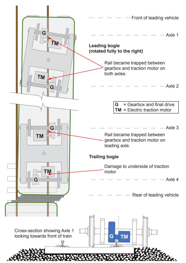
Figures 15a and b: Diagrams showing the leading vehicle of train 2K04 and interaction between traction equipment and right-hand rail during derailment. Figure 15b courtesy of RSSB.
