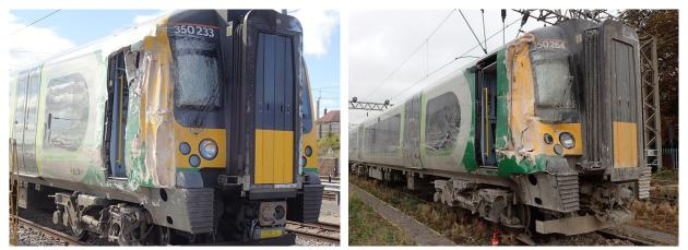
Figure 17a and b: Front view of train 2Y59 (unit 350233) and train 2K04 (unit 350264) following recovery from the tunnel
