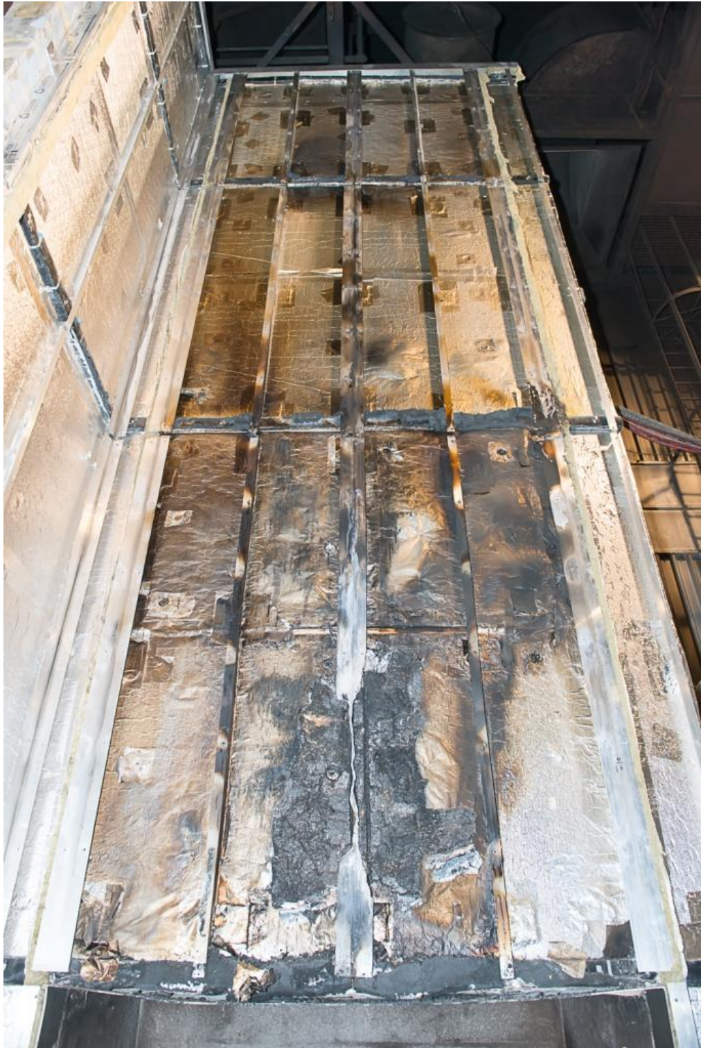
Figure 28. Damage to cladding system beneath ACM panels directly above the combustion chamber.
