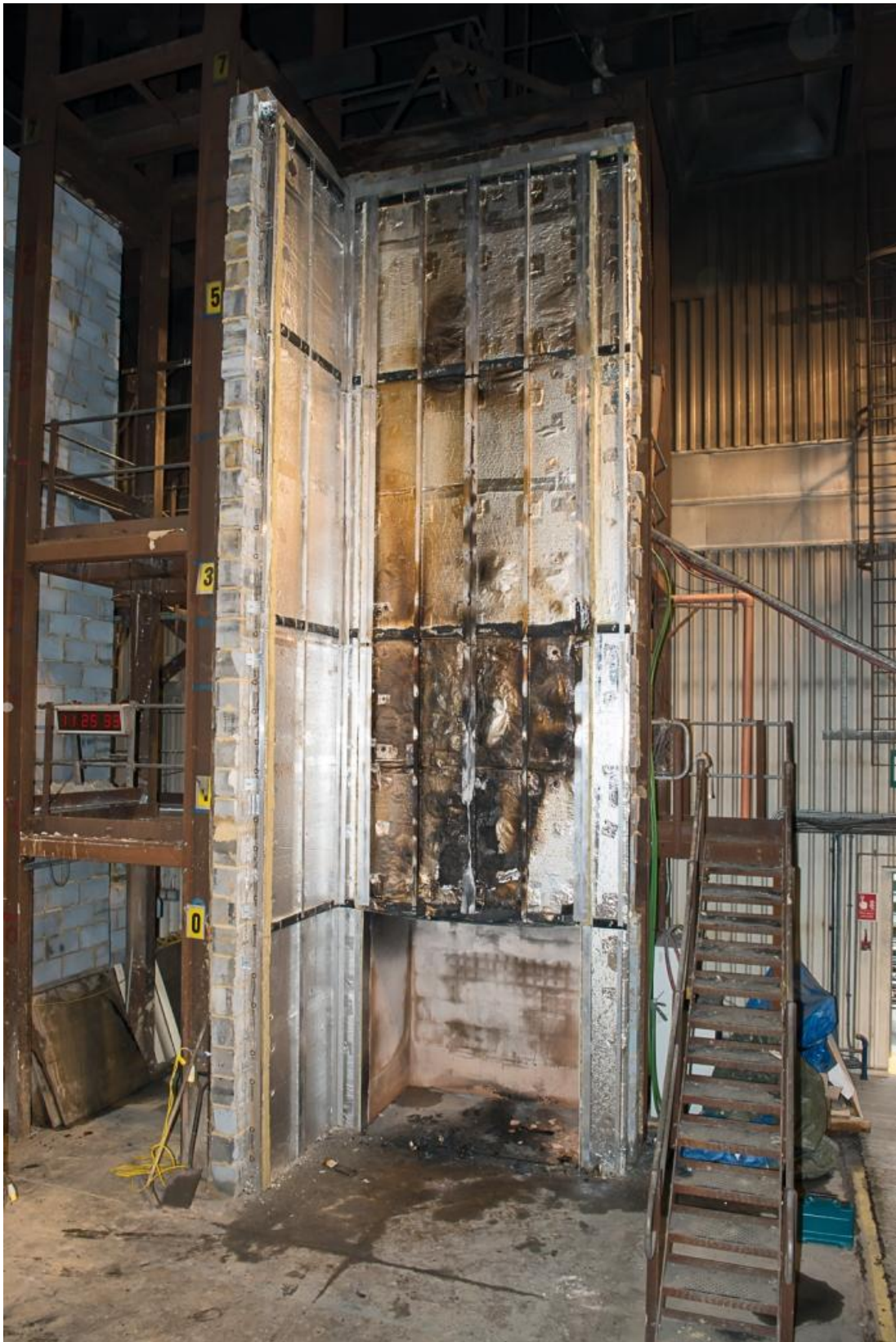
Figure 27. Full height photograph of system following removal of ACM panels.
