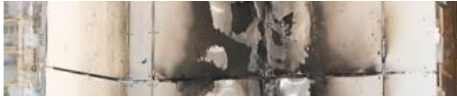
Figure 24. Zoomed view of discolouration on base of second row panels.
