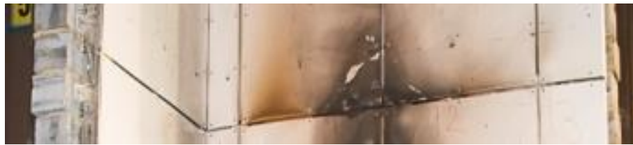
Figure 25. Zoomed of discolouration on base of third row panels.
