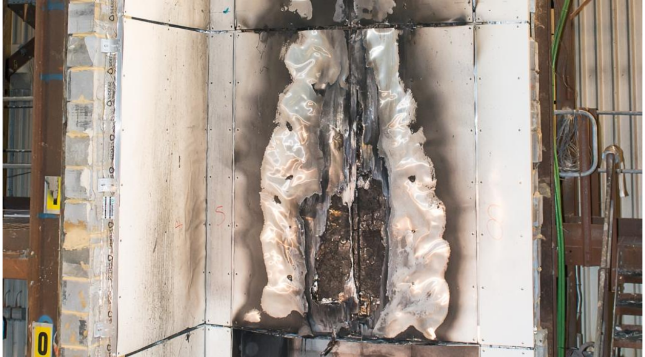
Figure 22. First row ACM panels (directly above combustion chamber).
