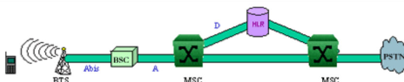
Figure 1. Simplified architecture of GSM
