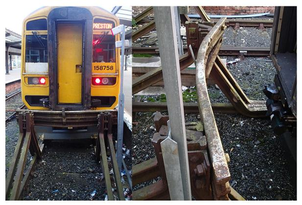
(Left) View of front of train with driving cab to the right of gangway; and (right) view of deformation in buffer stop beam after the collision
