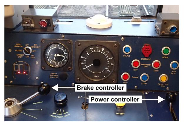
View of class 158 driver's desk showing power and brake controllers
