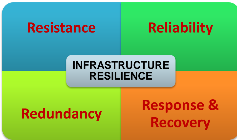
Figure 2: The components of infrastructure resilience: In building resilience, the contribution made by each of these four components needs to be considered
