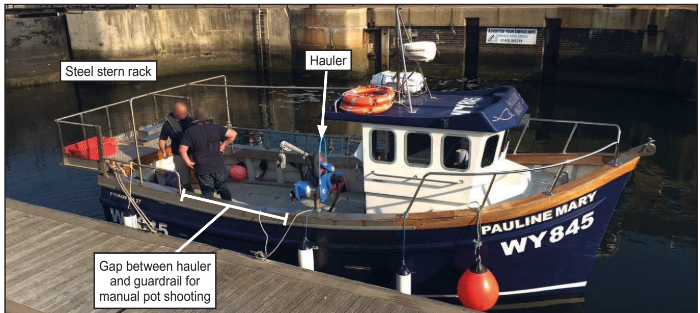
Figure 1: Pauline Mary showing deck layout and equipment
