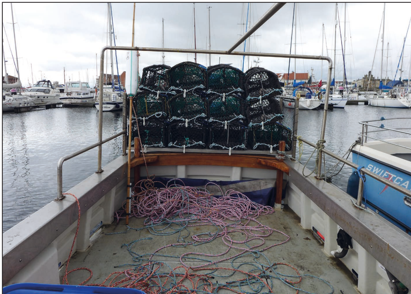
Figure 7: Illustration showing the final 12 pots on the stern rack, and the potential hazard associated with loose ropes on the deck
