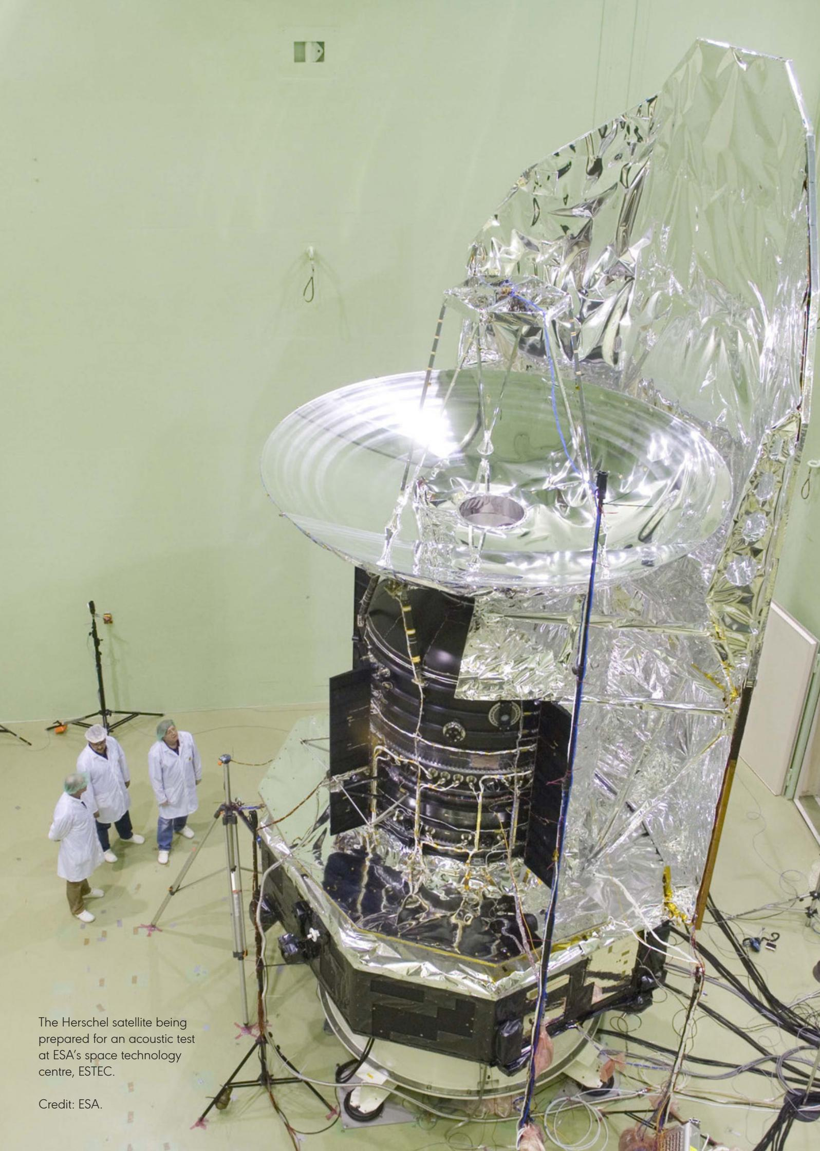
The Herschel satellite being prepared for an acoustic test at ESA's space technology centre, ESTEC.
