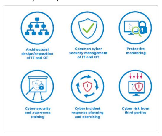
**Architectural design/separation of Information Technology (IT) and Operational Technology (OT)**: Ideally IT and OT systems or networks should be completely separated to prevent infections in IT systems spreading and impacting processes that could cause physical damage.
