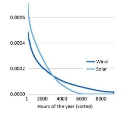
Figure 10. Generation duration curves for solar and wind power
