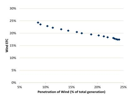
Figure 13. Capacity credit of wind assumed in the capacity market design
