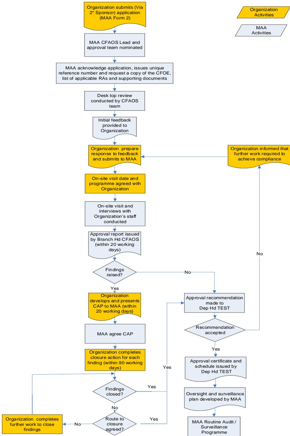
Figure 1 – CFAOS Initial Approval Process Flowchart
