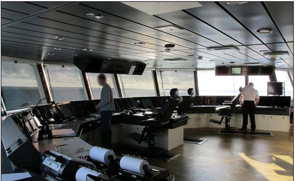
Figure 21: Example of another bridge with off-axis windows
