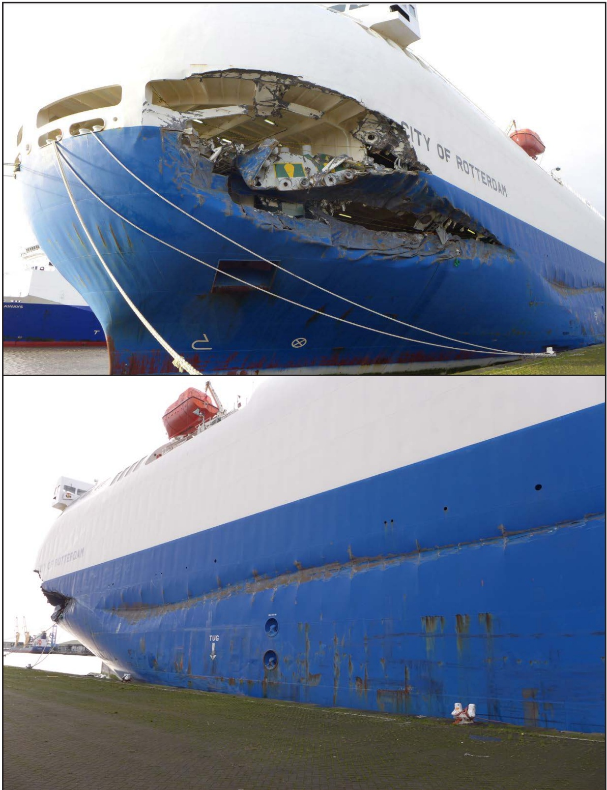
Figure 11: City of Rotterdam damage
