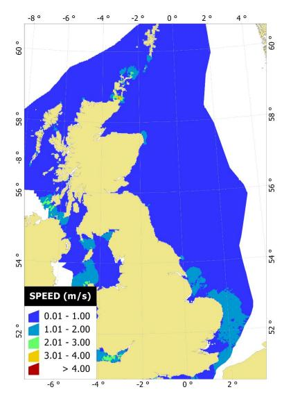
Figure 1. The peak current speeds on a mean spring tide (m/s) around the UK (Atlas of UK Marine Renewable Energy Resources 2008).
