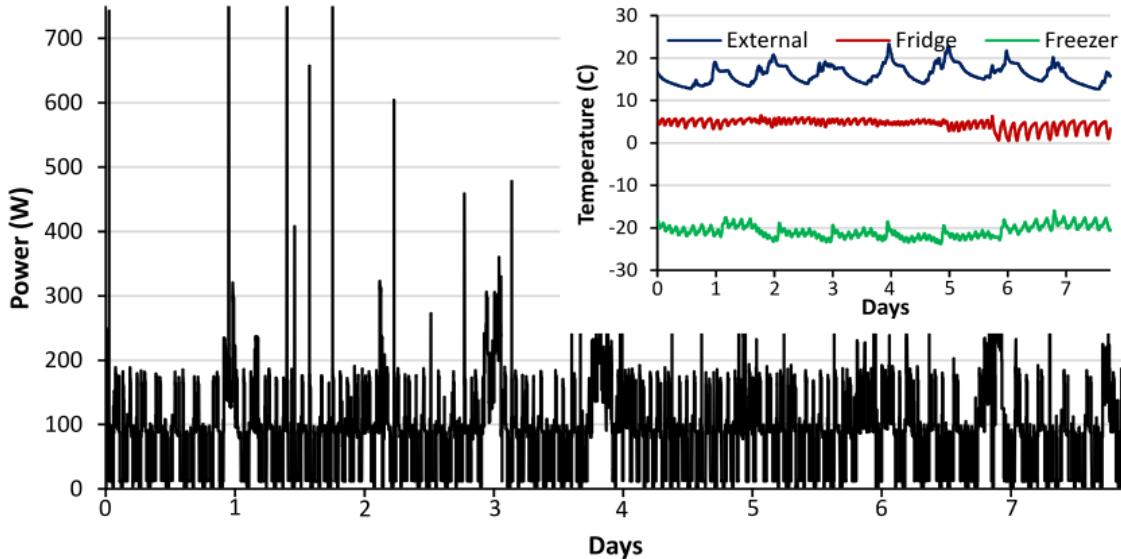
**Figure 35.** Electricity consumption and temperature, of a 'high' consuming, side-by-side appliance
