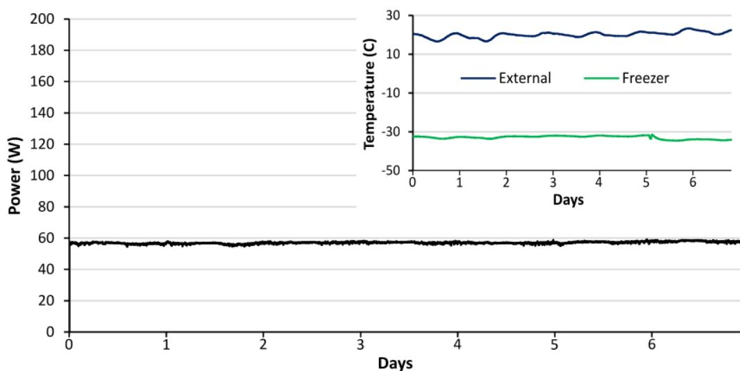
**Figure 36.** Electricity consumption and temperature, of an ‘over’-consuming appliance
