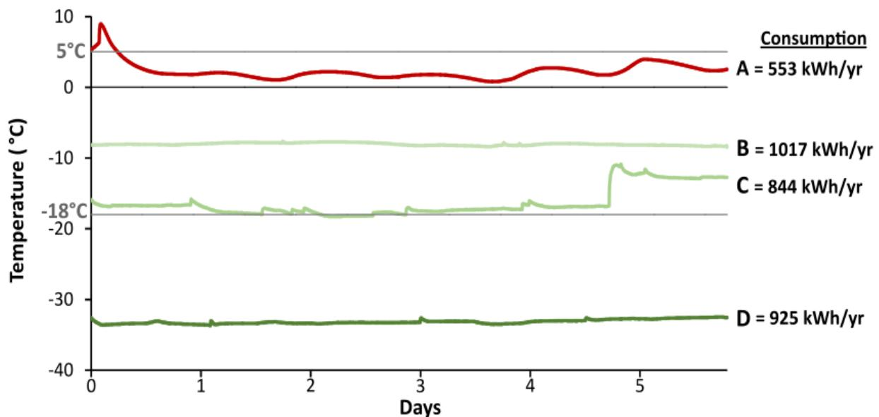
**Figure 37.** Temperature profiles of different over-consuming appliances (red = fridge, green = freezer), with reference lines showing recommended fridge and freezer temperature thresholds.
