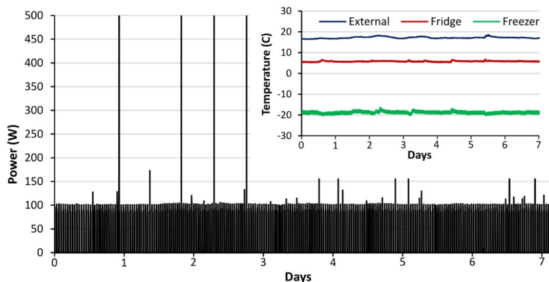
**Figure 33.** Electricity consumption and temperature, of a 'normal' appliance
