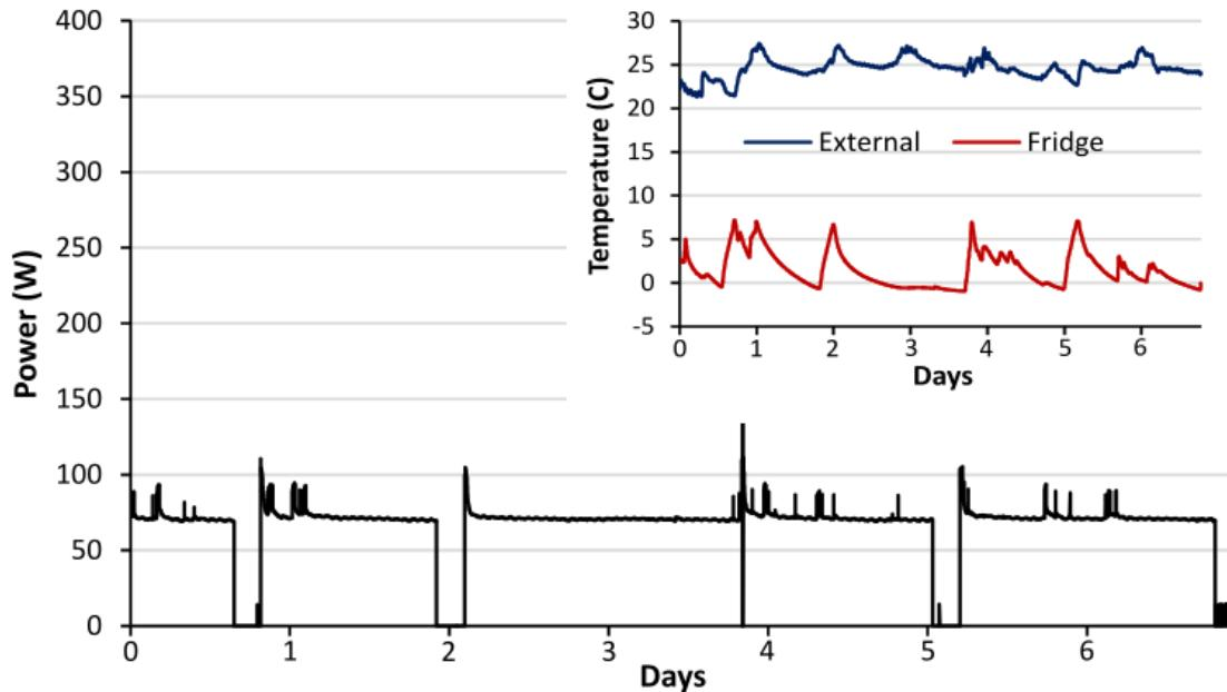
**Figure 38.** Electricity consumption and temperature, of an over-consuming appliance
