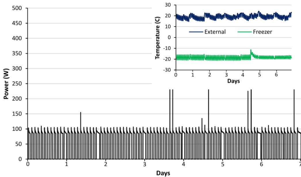
**Figure 34.** Electricity consumption and temperature, of a 'high' consuming appliance
