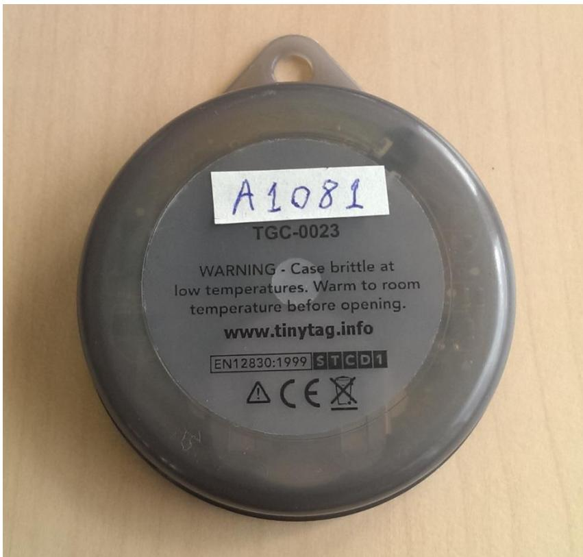
**Figure 2.** TinyTag transit 2 temperature logger.
