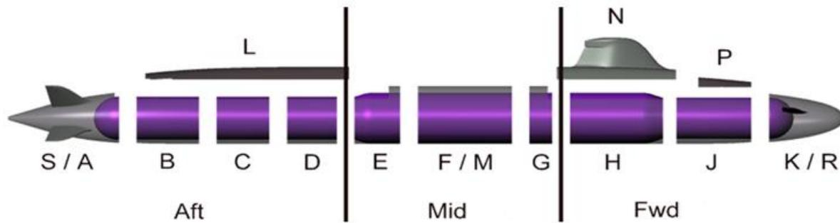
This modular approach shortens the overall build timescales. Manufacture and fabrication of the units begins in the New Assembly Shop. The units are painted and applied with acoustic coatings ready for the installation of the intricate systems and equipment in the Central Yard Complex. Finally, the units will pass to the existing Devonshire Dock Hall, to be combined to create mega-units, and mega-units are then combined to form the submarine.
