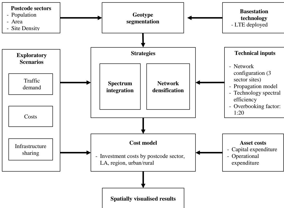
In order to assess deployment costs across Britain, the approach used in this study groups areas that have similar cost characteristics together into specific geotypes. The key cost characteristics include population density and existing site density. Once these geotypes have been defined, network dimensioning is undertaken using the key parameters for each geotype segment.
