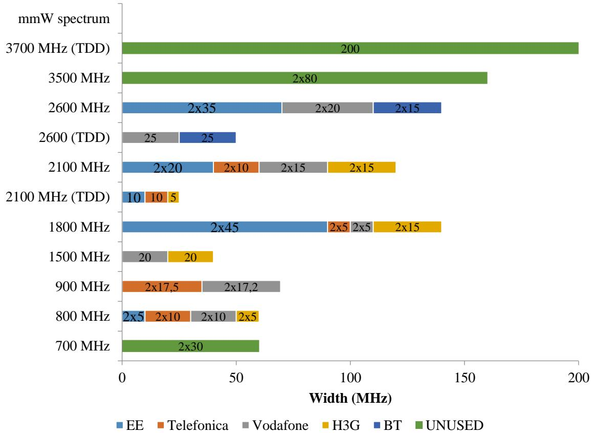
In addition, 900 MHz and 2100 MHz are excluded from the current analysis as 2G and 3G networks operate on that spectrum. Although a ‘refarming’ process might be expected in the long-term, at this point we do not have any evidence to suggest that these bands will be available for future rollout during the period examined in this study.
