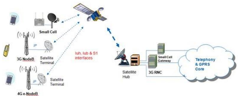
Figure 38: Use of satellite in cellular networks
