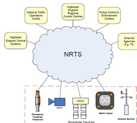
In terms of future opportunity, Highways England (HE) network is made up of a number of different fibre deployments ranging from legacy 1990s 12/24 core to 96 core fibre installed on the newest smart motorways sections of road. Depending on location there are levels of unused dark fibres with most capacity on the smart motorways sections, hence older deployments between 1990 and 2009 in lesser demanding areas of the network have reduced fibre capability.
