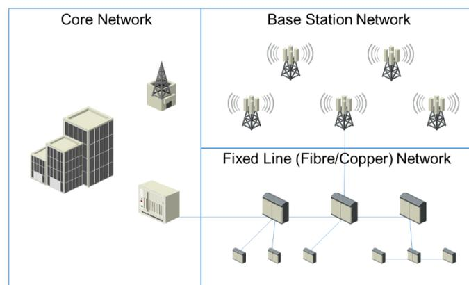
Figure 15: Simplified Private Radio/Fixed network architecture
