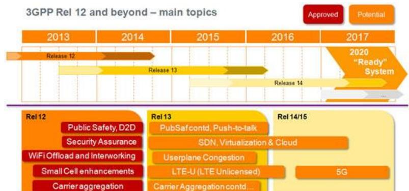
Figure 37: Standardisation timeline for SDN/NFV
