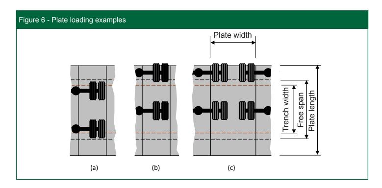
stress is still likely to occur when the lighter half-axle is off the span and the heavier half-axle is at mid span (and at its edge) - see Figure 6b. Plates a little over 1.25 m wide can be loaded by half-axles from two adjacent vehicles, as shown in Figure 6c.
