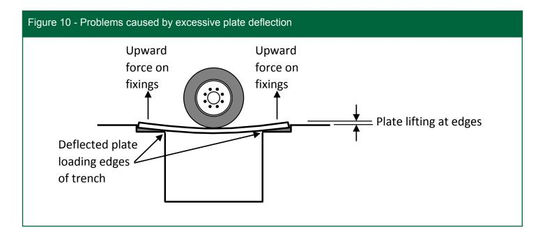
to remove as they might turn but not unscrew. Where speedy removal is essential after plates have been in place for some time, it is important that the fixings do not hinder the process. If there is any doubt about the fixings, it may be necessary to check that they can be removed, say, 24 hours before they need to be.
