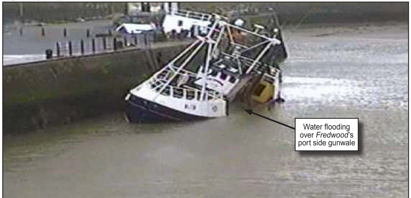
Figure 4: Maryport harbour CCTV snapshot of Fredwood at 0822 on 6 April 2016
