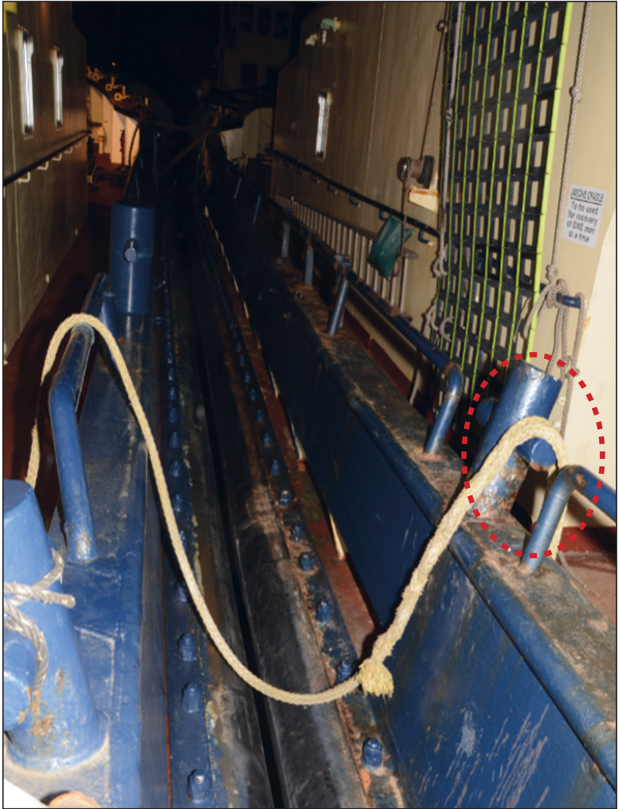
Figure 3: Amidships mooring rope as found following accident (reconstruction)
