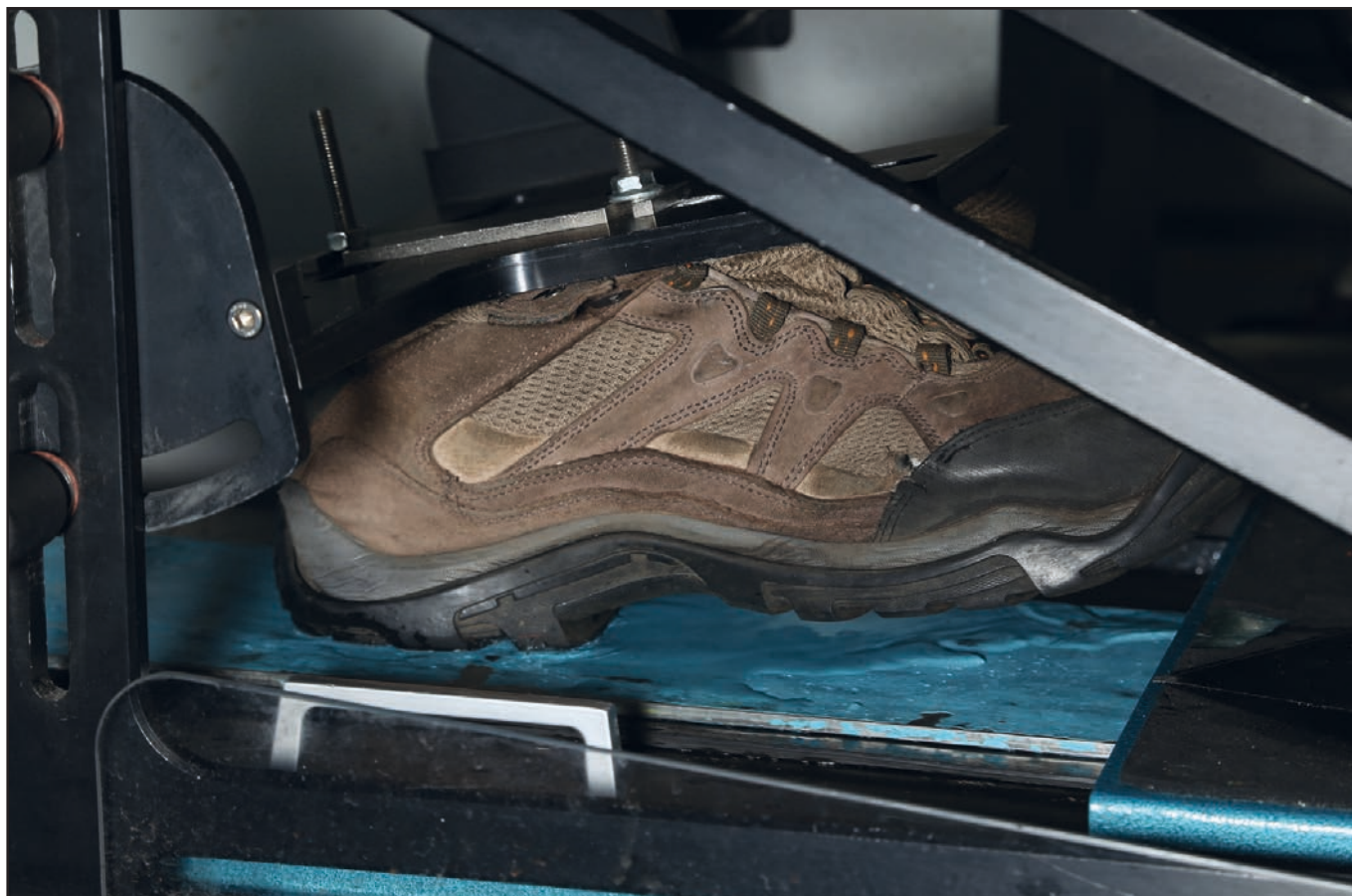
Figure 5: Walking boot undergoing slip resistance testing
