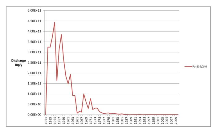
Figure 5.3 Annual aerial discharges from the Sellafield site – plutonium-239/240 (high stack)
