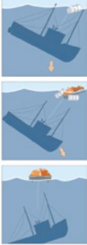
1. If vessel sinks, Hydrostatic Release Unit activates and liferaft attempts to float to surface
