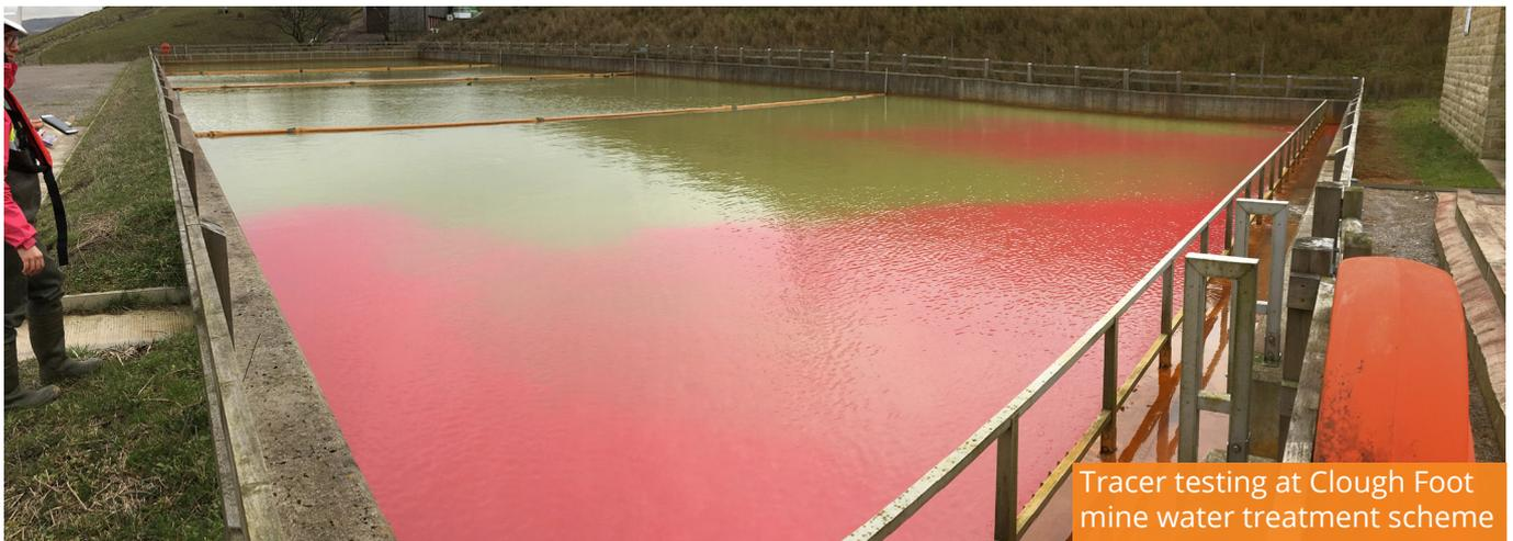
Tracer testing at Clough Foot mine water treatment scheme
