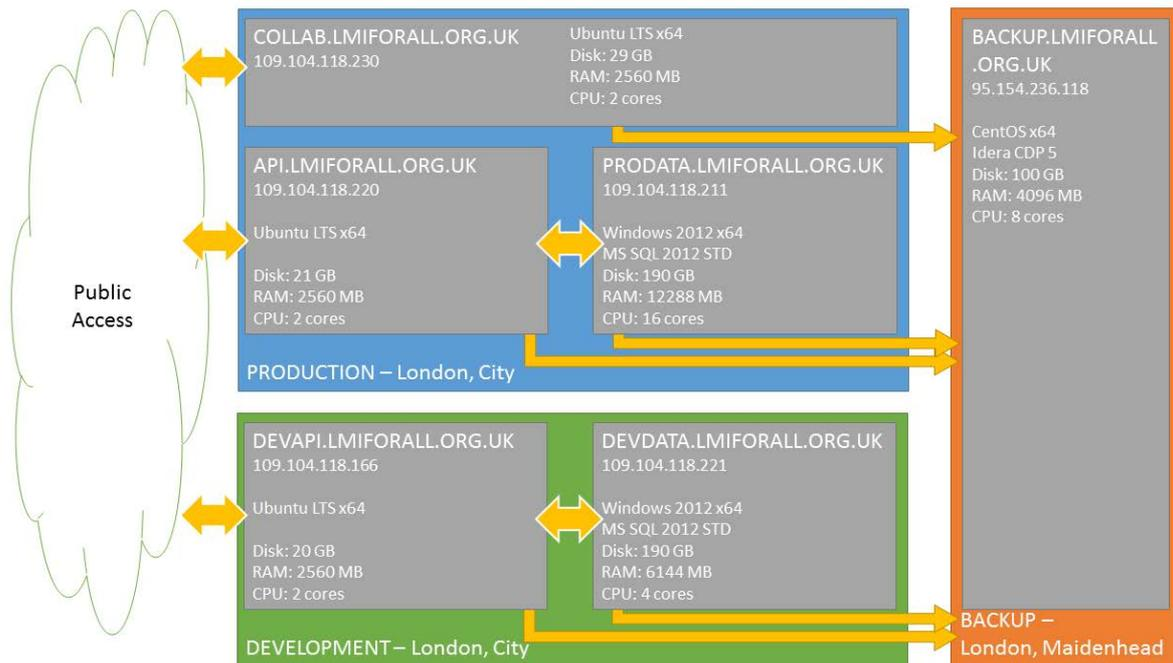
The development environment contains exact copies of the API and PRODATA servers in the production environment and is being used to develop and test new functionality and data-updates before they go live in production. Below is an overview of the two database servers.
