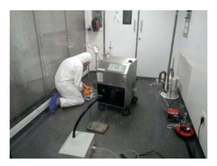
Biosafety staff undertake sampling of a heater cooler unit under controlled and reproducible laboratory conditions to assess the aerobiological risk
