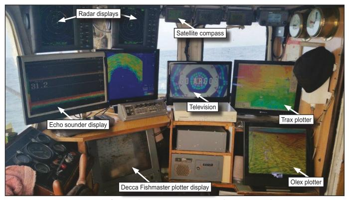
**Figure 6:** *St Apollo*'s wheelhouse equipment (starboard side)
