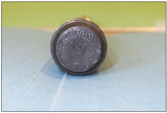
Figure 20: Grade marking on the M24 tie bolt
