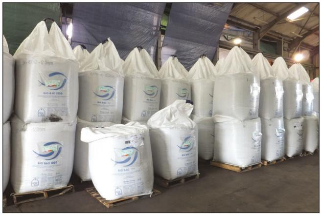
Figure 19: 1 tonne Flexible Intermediate Bulk Containers (FIBC)
