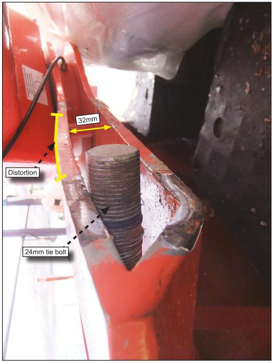
Figure 12: A 24mm tie bolt through a 32mm slot (inboard side)
