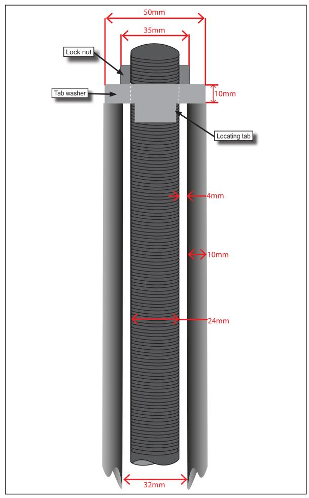
Figure 24: Diagram showing the tab washer arrangement
