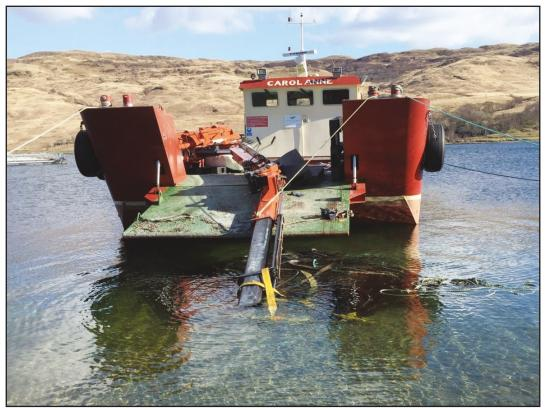
Figure 4: Collapsed crane
