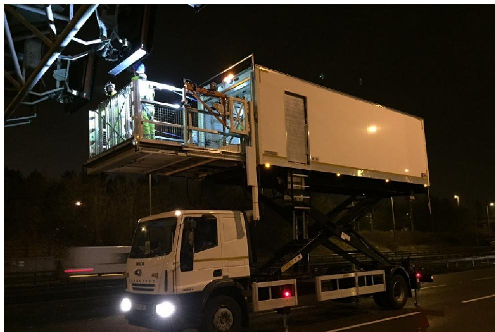
The Maintenance Assistance Vehicle (MAV) is the brainchild of Professional & Technical Solutions and is being taken forward as an innovative solution to address the ongoing maintenance and servicing of signals. The vehicle provides a safer, quicker way for road workers to replace overhead, electronic gantry signs; providing a safer environment for road workers while they work inside the vehicle - and on a sturdy platform while they work outside.
