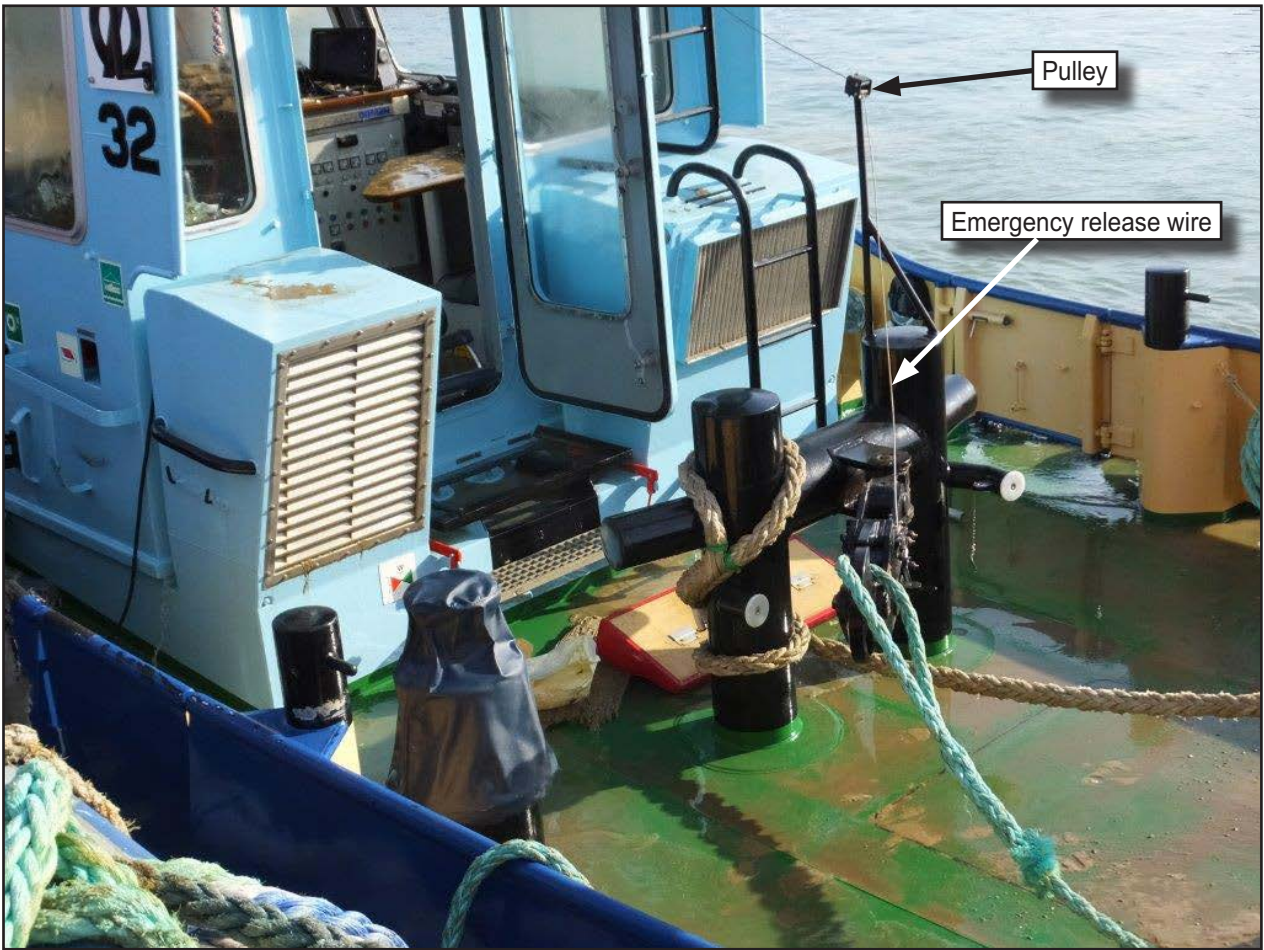
Figure 9: Towing hook emergency release wire
