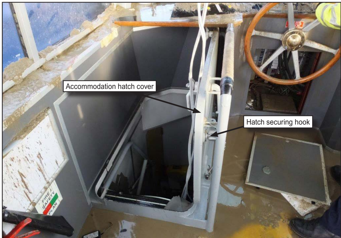
Figure 4: Accommodation hatch cover (hooked open)
