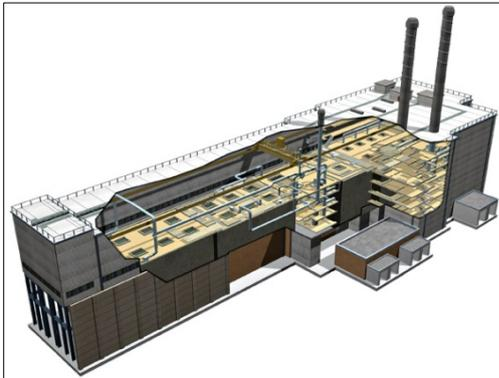
The Magnox Swarf Storage Silos (MSSS) is one of four facilities at Sellafield known collectively as the Legacy Pond and Silos. We are focused on safely decommissioning these buildings as part of our hazard and risk reduction programme.
