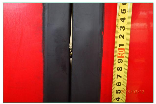
Figure 7: Zip slider, as found in door showing height above train floor
