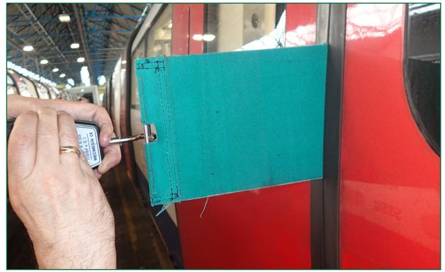
Figure 14: Pull-out testing with canvas piece
