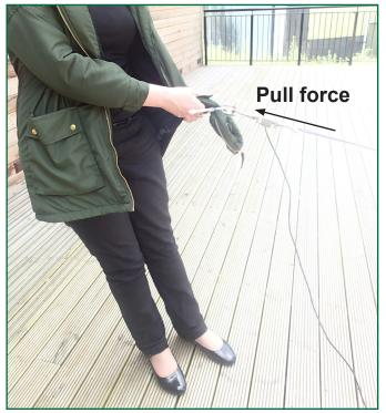
*Figure 12: Testing pull-out force applied by person wearing incident coat*
