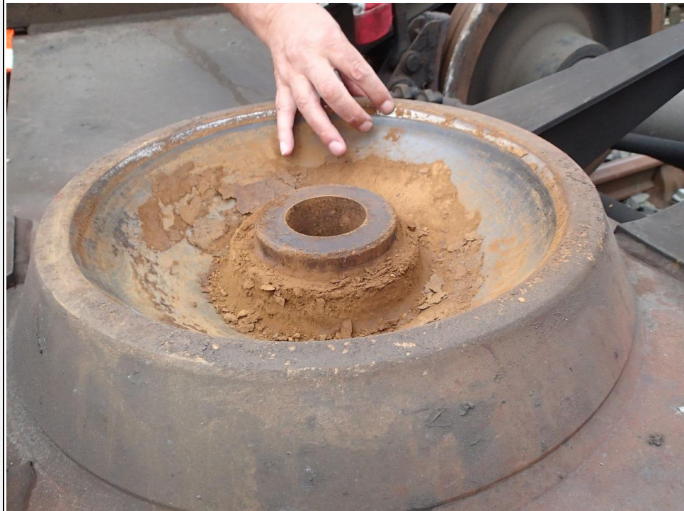
Figure 2: Centre pivot liner worn below level of steel rim, leading to contact between steel surfaces
