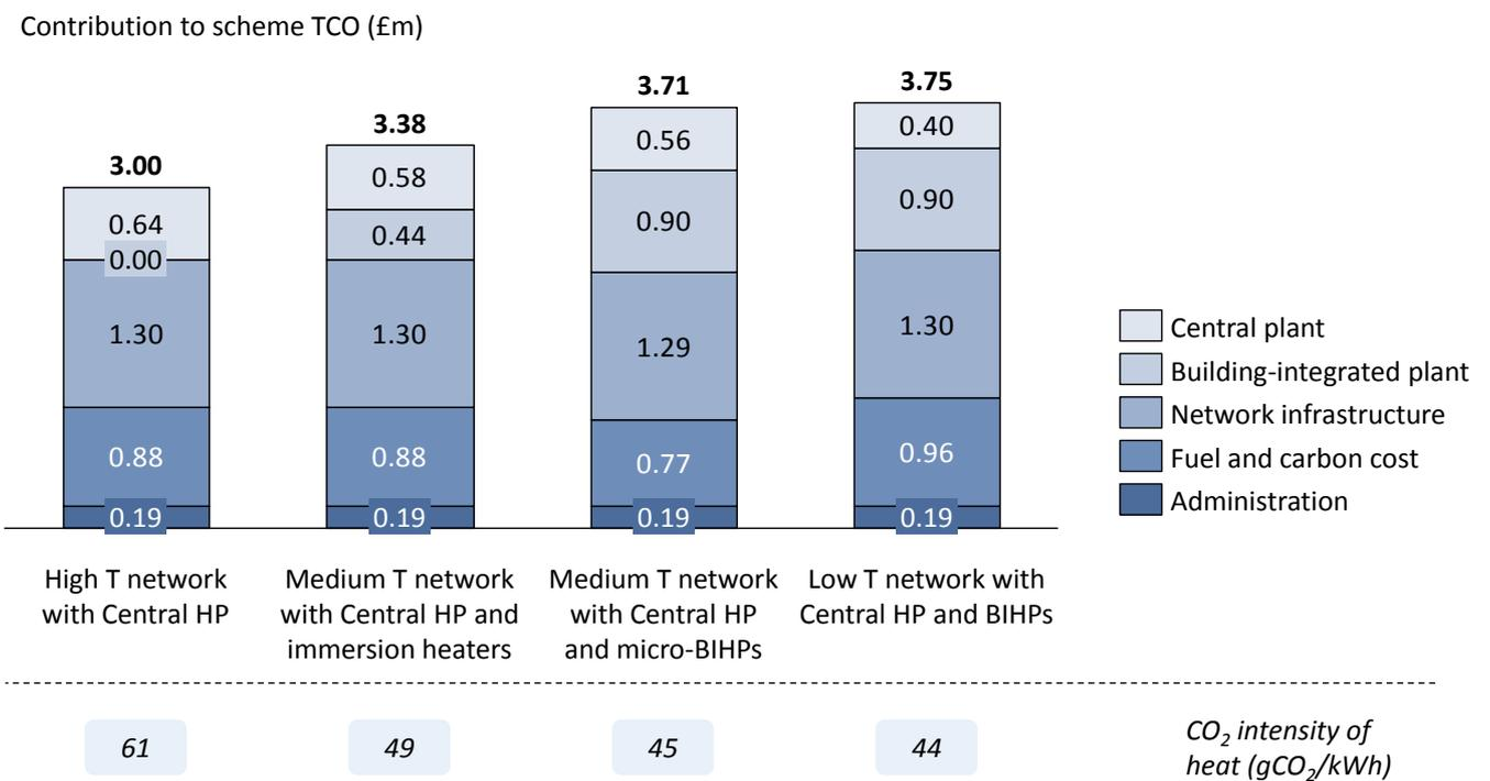
**Figure 7: Summary of TCO and CO<sub>2</sub> intensity of heat for the two HP in DH configurations studied for Demand Case B, a large-scale mixed-use development of existing buildings.**
