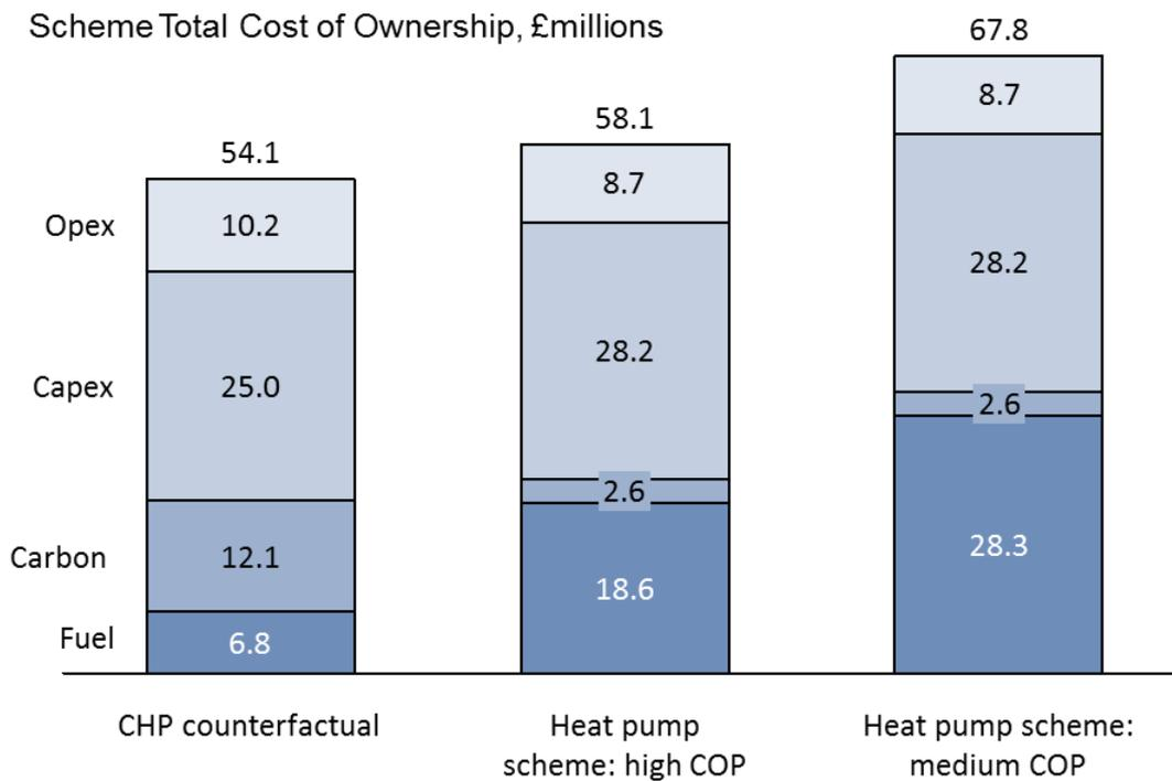
Figure 50 shows the TCO breakdown of the counterfactual and two heat pump schemes. Please note that the 'fuel' component of the chart is the resultant of positive cost of gas and electricity and the revenue (negative cost) from electricity generated by the CHP.
