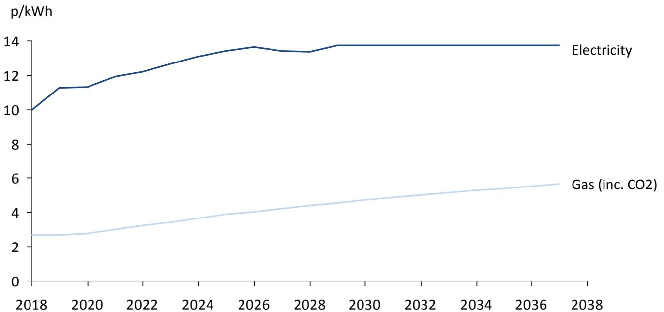
Given the average electricity/gas price ratio over the 20-year period in consideration, and the efficiency of gas-based counterfactual heating plant, it is possible to calculate the minimum COP of a heat pump which beats a boiler or CHP counterfactual on fuel cost:
