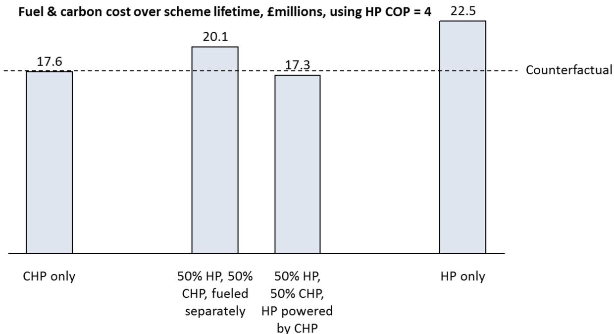
Figure 52 shows the same four configurations, but using a higher COP. This time, using CHP electricity to power the heat pump has led to lower running costs overall.
