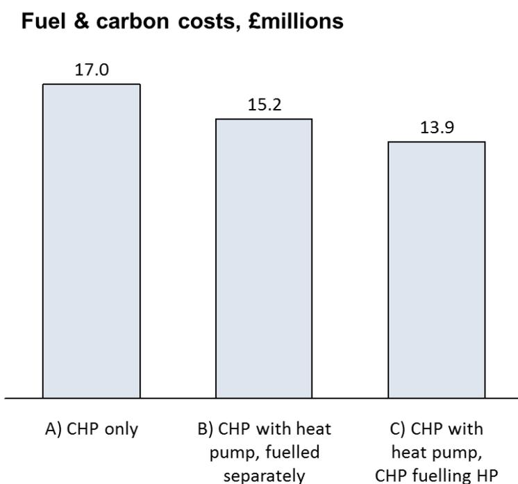
The fuel/carbon cost saving achieved by carrying out half of the heating using heat pumps, although noticeable in Figure 53, is not dramatic as might be expected from use of a heat pump
