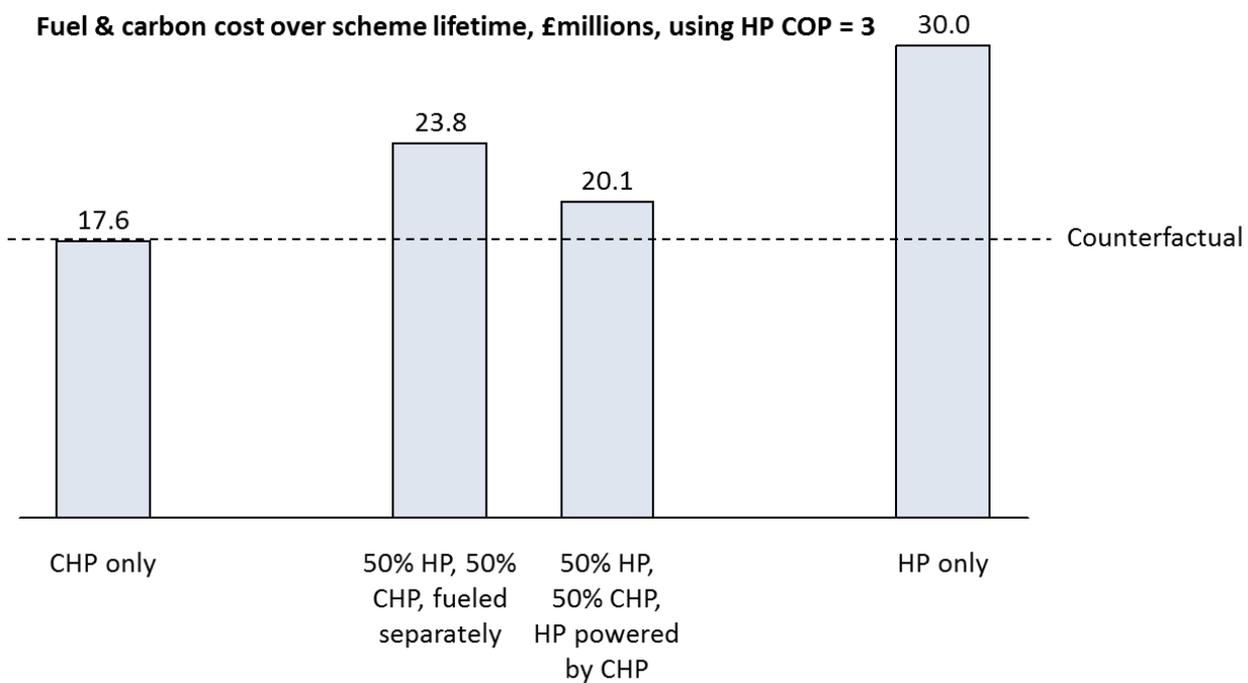
Figure 51 illustrates the effect of this strategy on total fuel & carbon cost. It can be seen that using CHP electricity to power the heat pump does indeed lower the fuel cost, but at a heat pump COP of 3, the lowest fuel & carbon cost is still achieved by the CHP only system.
