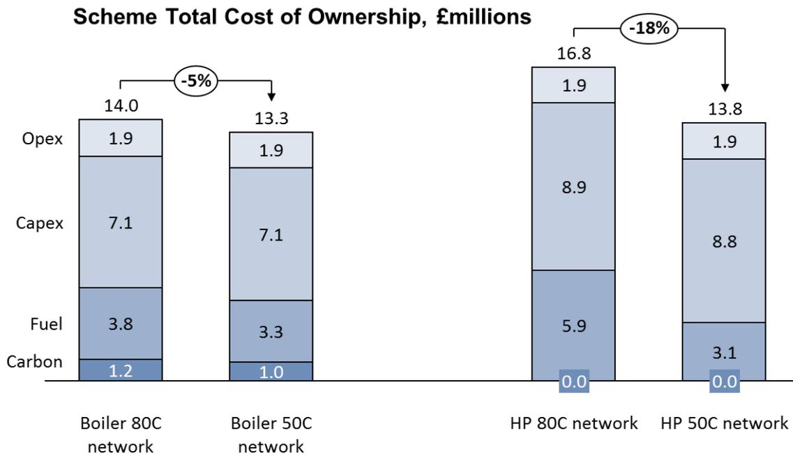
It is clear that in heat pump schemes, delivering heat at as low a temperature as possible is desirable for cost reduction, mostly to improve the heat pump performance. The next two sections will explore different ways of achieving the required space heating and DHW temperatures in the context of lower temperature networks.
