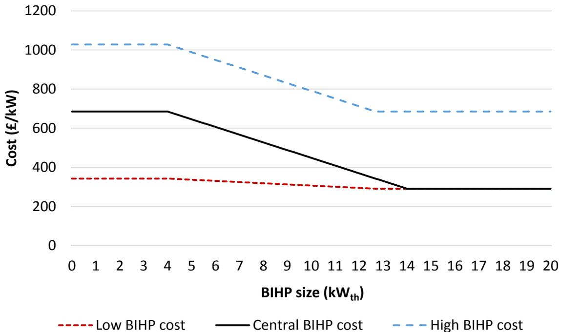
It can be seen from Table 6 and Figure 9 that, for the majority of the sensitivity assumptions, the cost presented for the central heat pump is greater than that for the building-integrated heat pump on a per kW basis. This may be surprising given that, as shown in Figure 9, the cost of building-integrated heat pumps decreases with increasing capacity on a per kW basis. There are three factors contributing to this:
