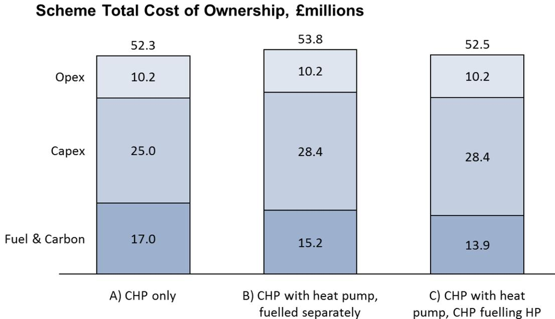
Figure 54 shows the scheme total cost of ownership for the three configurations. Please note that ‘opex’, or operating cost, has been set to constant; in general heat pumps are less costly to maintain than CHP<sup>40</sup> but in this case the complexity of the heating plant has been increased by fitting a heat pump onto a CHP, so it was judged that there should be no reduction in operating costs.
