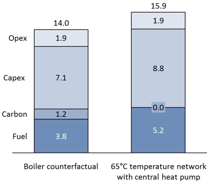
To decrease the running cost of the heat pump scheme, we wish to further reduce the network temperature. Rather than lowering this to ambient temperature and upgrading its heat using building-scale heat pumps to provide the space heating and hot water, an alternative strategy is to use the network to provide space heating and minimal building-scale plant to upgrade this heat to that required for DHW.
