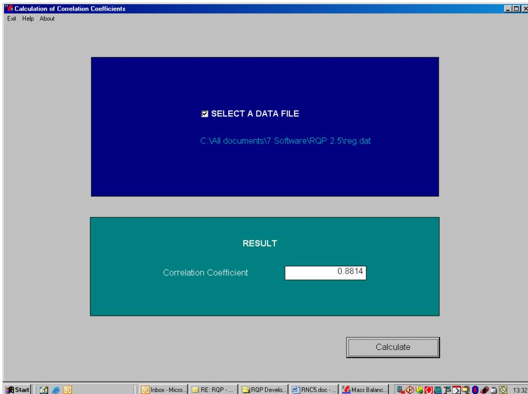
The data-file consists of pairs of values of the variables for which you want to calculate the correlation coefficient. REG.DAT has the 12 rows of data shown below. In the first row, for example, the values 2 and 4, could be corresponding values of discharge flow and river flow - values measured at the same time.
