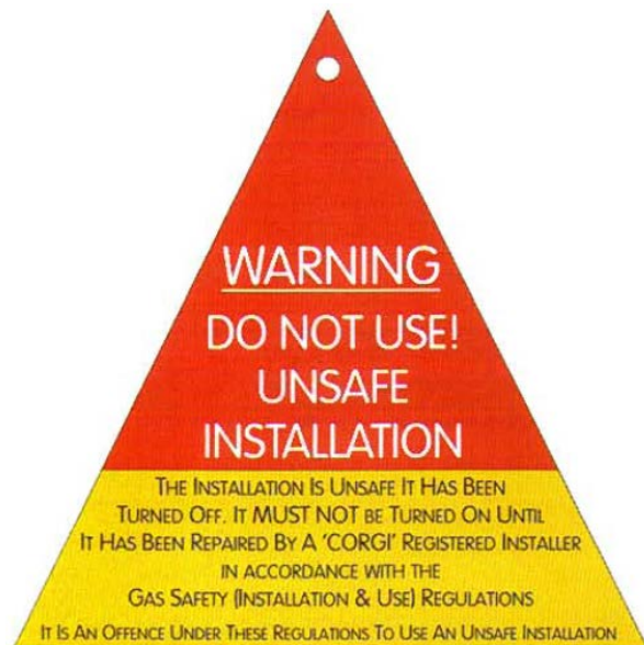
WSG2 – Unsafe Installation Warning Label
