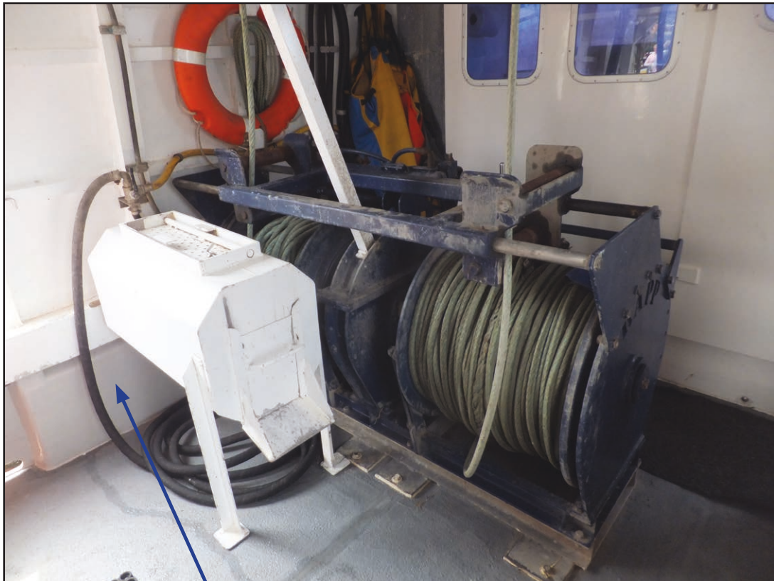
Figure 11: Position of port side engine room air intakes between bulwark frames
