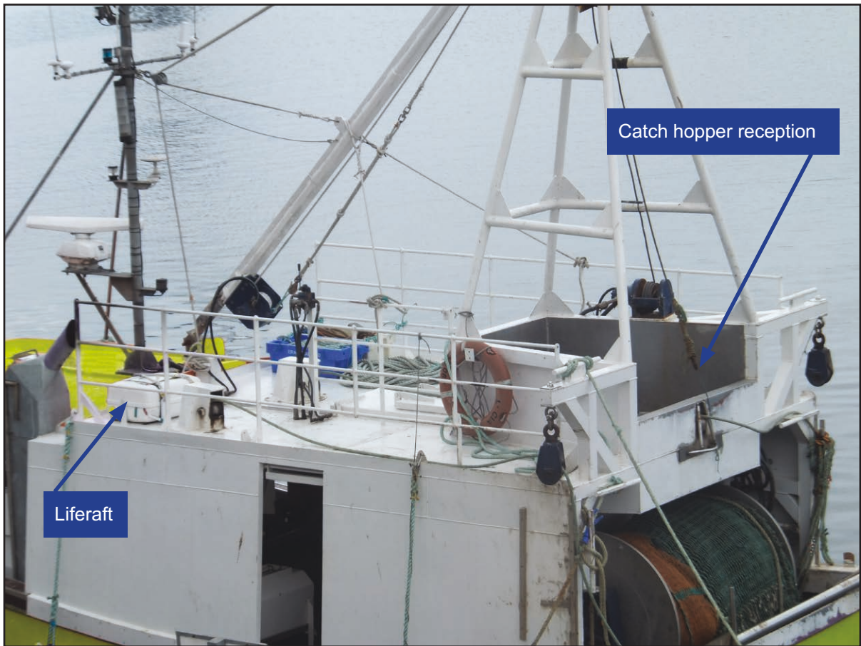
Figure 12: Position of catch hopper below gantry
