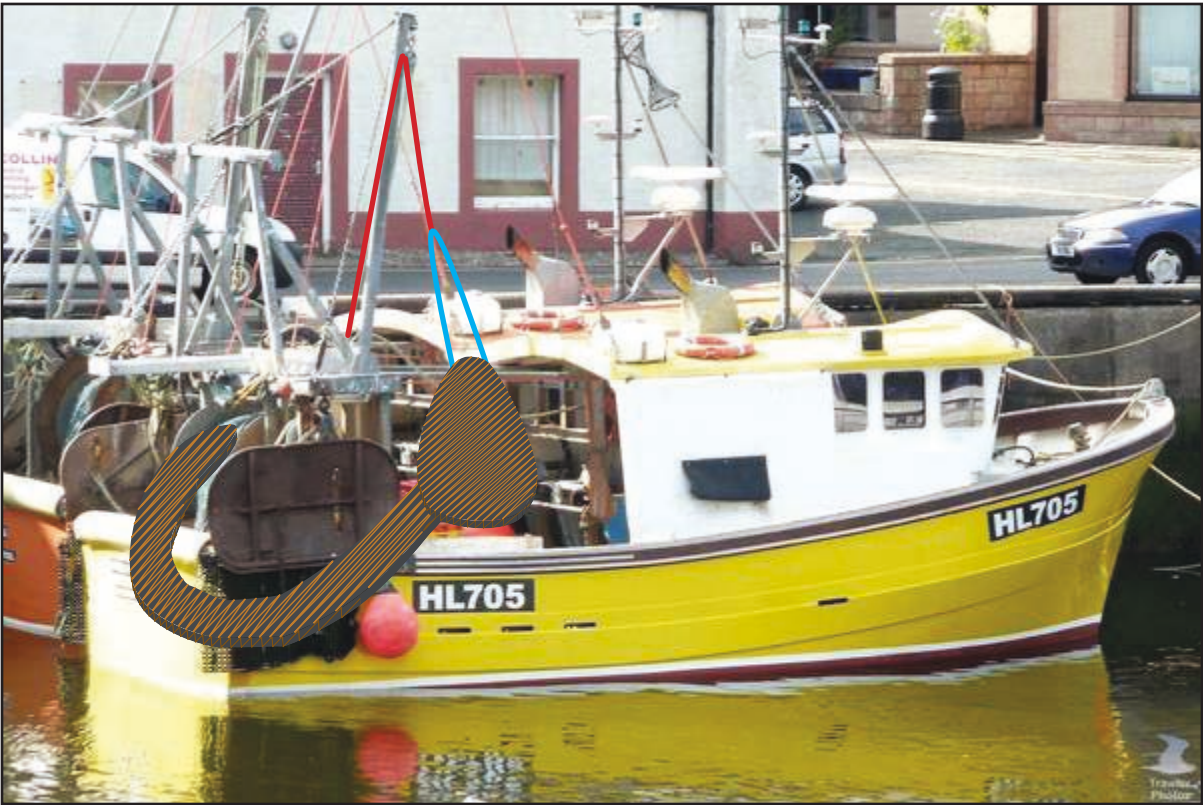
Figure 14: Depiction of cod end being hoisted over the side of the vessel before modernisation
