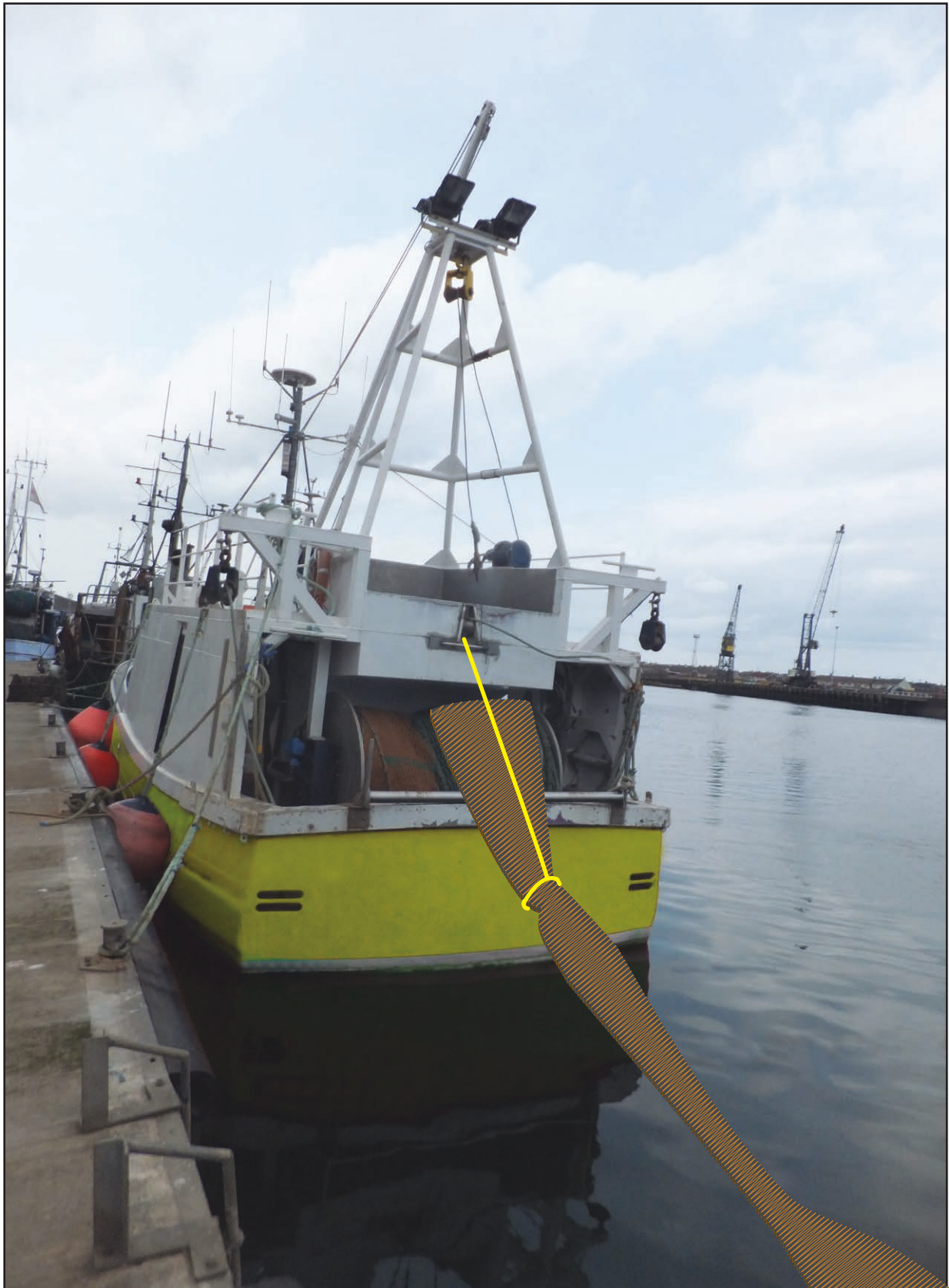
Figure 3: Depiction of cod end being towed to wash out mud
