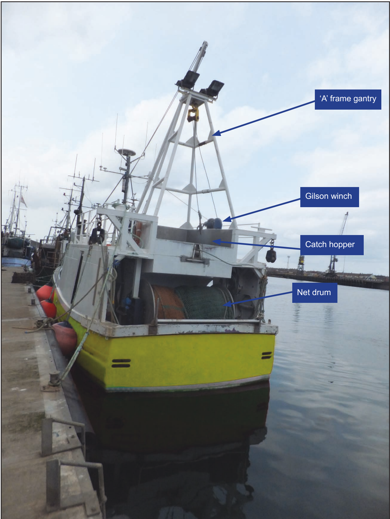
Figure 2: Net drum and gantry arrangement
