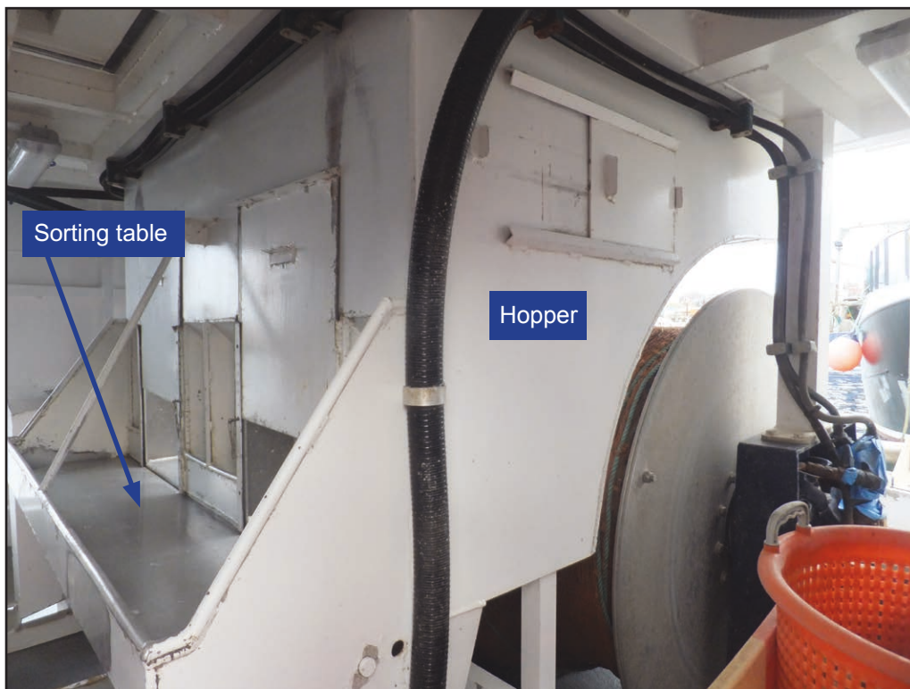
Figure 13: Catch hopper on main deck
