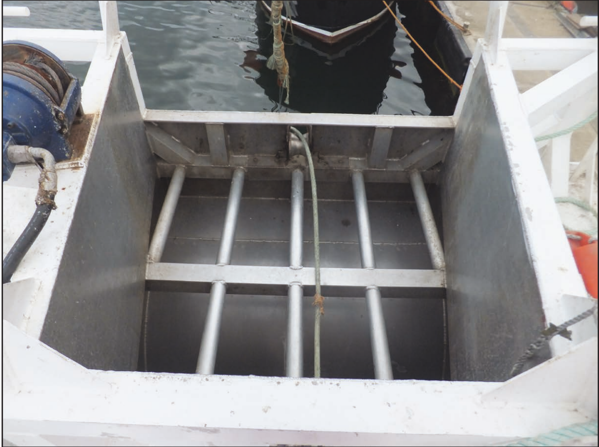
Figure 17: Catch hopper seen from above
