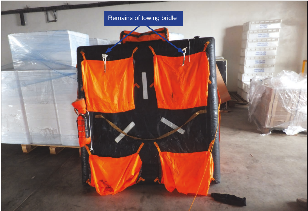
Figure 9: Stella Maris liferaft showing remains of towing bridle
