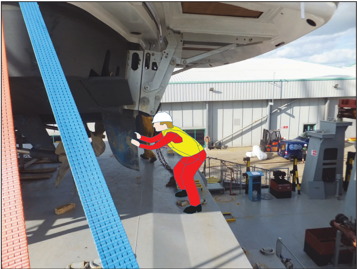
Figure 3: Position of the chief officer as he checked and adjusted the alignment of the yacht's keel
