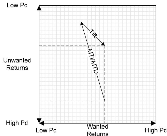
The reason that MTI/MTD succeeds where simpler techniques fail is the exploitation of a difference in what Skolnik refers to as the “character” of the unwanted echoes when compared to the wanted echoes. It is only through exploiting the character differences between turbine and aircraft echoes that turbine returns can be safely ignored without impacting aircraft detection.
