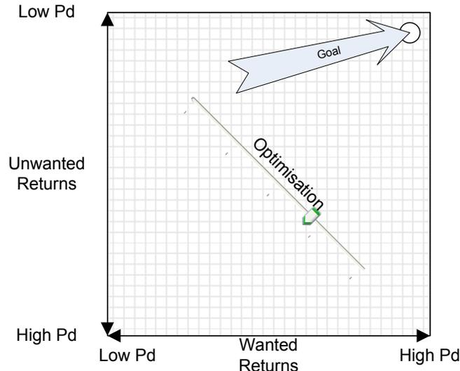
Moving target indication, MTI, and its subsequent evolution into moving target detection, MTD, was the radar design breakthrough allowing the greatest step towards the goal of detection without clutter. Although MTI reduces the  $p_d$  of unwanted returns only at the expense of wanted returns it uses the instantaneous radial velocity of the reflecting object to weight this reduction in favour of removing returns from stationary objects.
