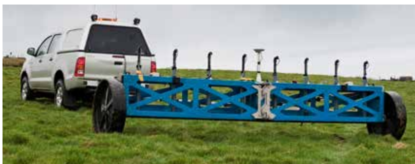
DIO EOC magnetometer array used to detect ferrous anomalies in the ground © Crown
