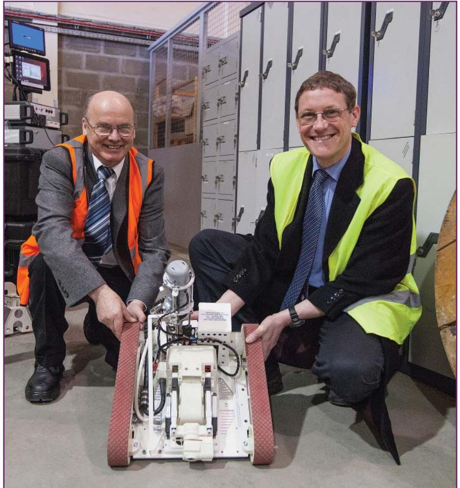
The WallRover, a lightweight, remotely operated vehicle (ROV), that can climb walls, was developed by Dr Gary Sewell, with manufacturing partner Smith Engineering (GB) Ltd.
