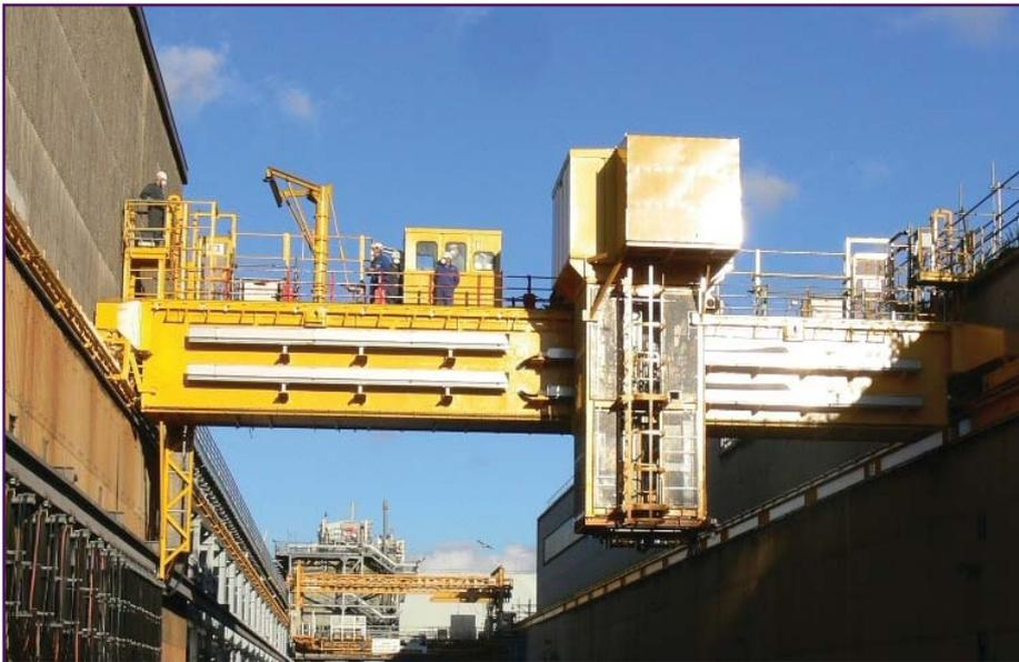
The 60-tonne crane, known as the skip handler, straddles the First Generation Magnox Storage Pond (FGMSP) and is used to move skips of spent fuel, waste and equipment around the open-air pond. It is also a critical element in the programme to retrieve and treat the pond's radioactive contents.
