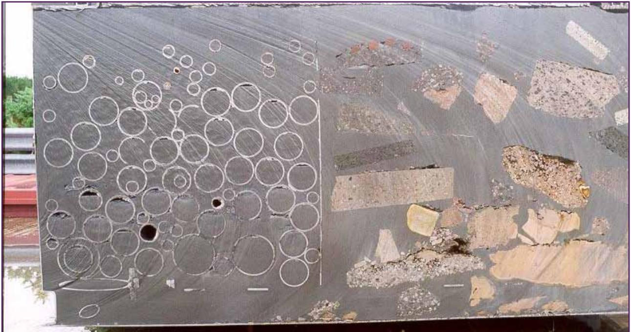
**Waste is grouted with a cement mix before being placed in vault**
