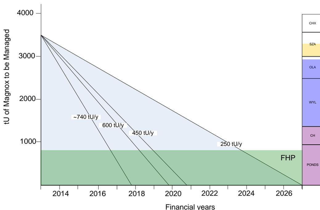
Figure 2: Schematic illustration of the quantity and location of Magnox fuel as a function of MOP performance (CHX: Chapelcross, SZA: Sizewell A, OLA: Oldbury, WYL: Wylfa, CH: Calder Hall)
