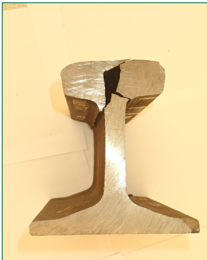
Figure 13: Cross-section of rail showing extent of VLS
