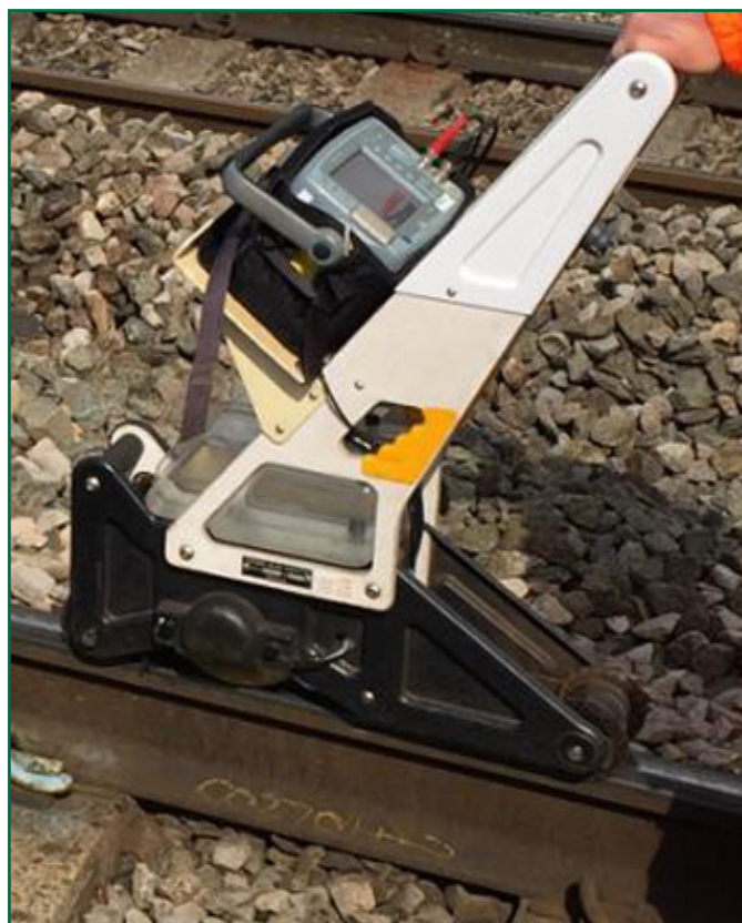
Figure 8: Sperry ultrasonic 'walking stick'
