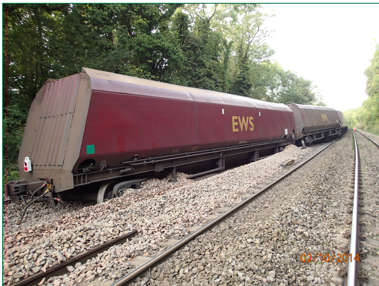
Figure 4: Derailed HTA wagon
