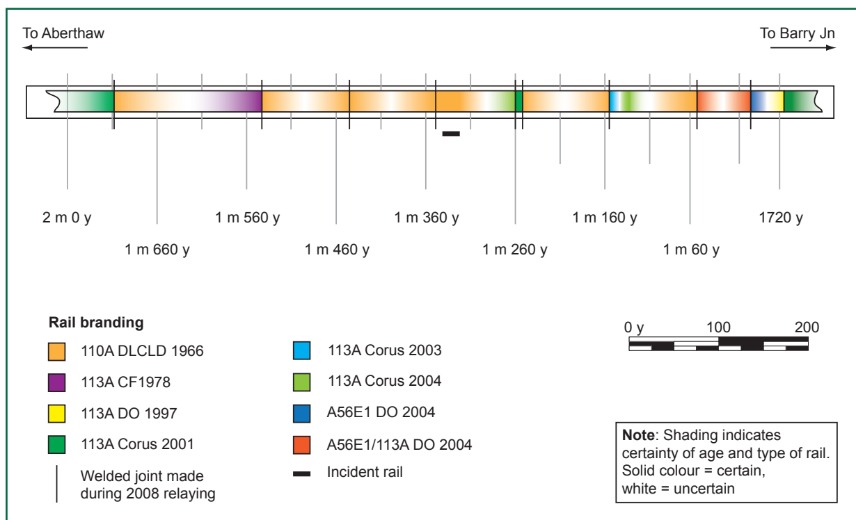
Figure 14: Plan of left-hand rail at Porthkerry showing rail type and age
